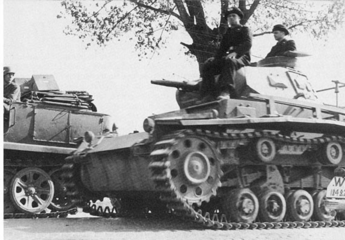
A PzBefWg III Ausf D1 passes an eighteen ton tractor on a road in Poland. The complex leaf suspension system of the Ausf D1 was less than satisfactory and these vehicles were quickly withdrawn from service during 1941.
