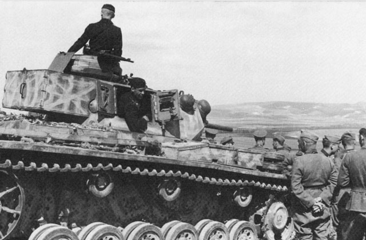
This PzKpfw III Ausf J, believed to be of 1.PzDiv is fitted with a non-standard turret stowage bin similar to those seen on earlier PzKpfw III Ausf Hs. The Dark Gray camouflage has been overpainted with a hand brushed pattern of Dark Yellow.
