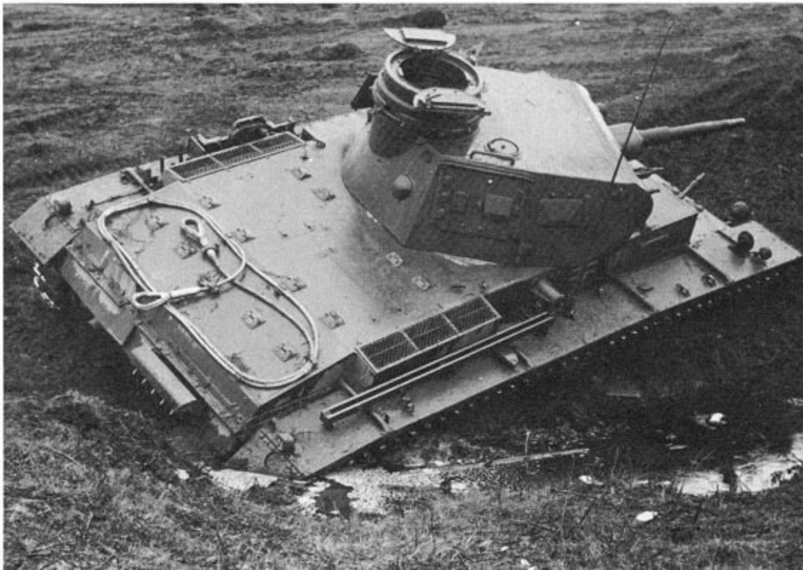
A PzKpfw III Ausf E has slid into a water filled shell hole and become bogged down. The screened over boxes on either side of the rear engine deck are the engine air intakes. The box on the starboard side of the tailplate houses smoke candles which could be released singly or in salvo.
