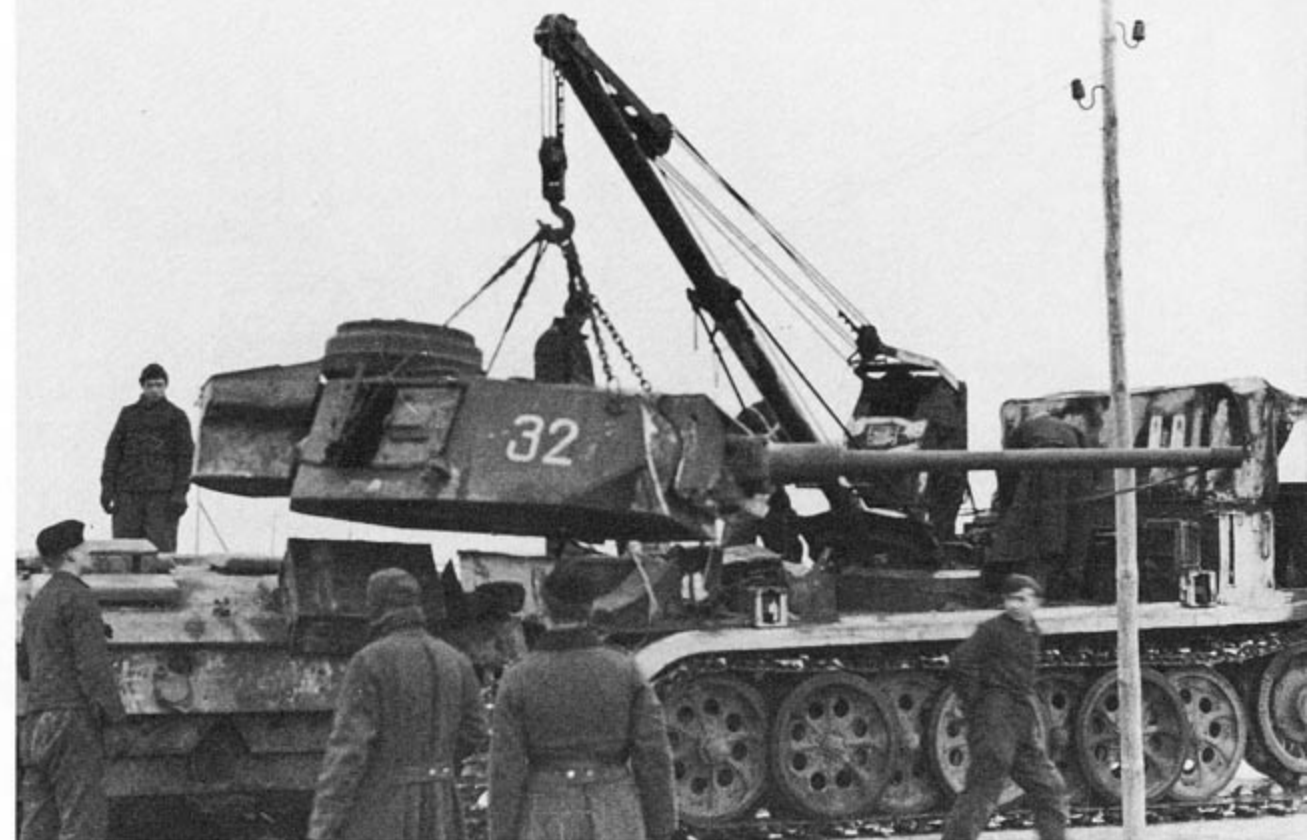
Although badly damaged tanks were usually sent to overhaul depots for major repairs, it was not uncommon for field repair shops to rebuild as many vehicles as possible. Sub-assemblies could be exchanged between tanks allowing parts from seriously damaged tanks to be easily salvaged for use in repairing other vehicles.
