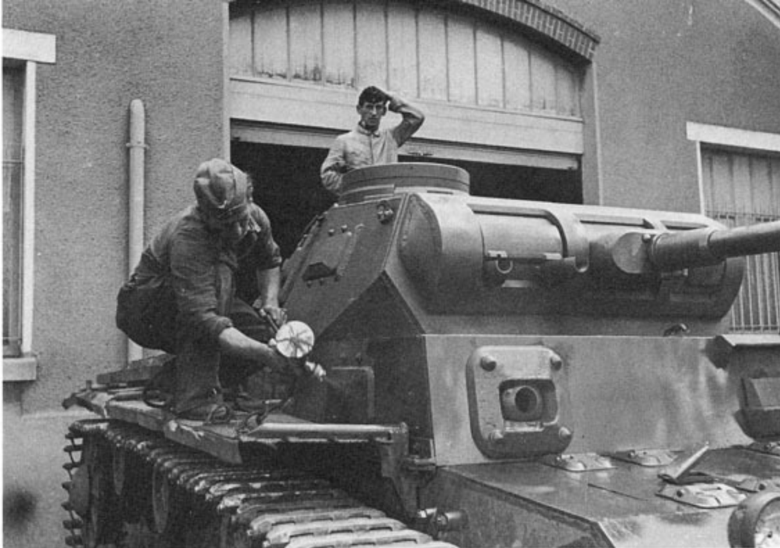
Maintenance personnel apply a fresh coat of paint to a PzKpfw III Ausf E. The vision block above the armor sleeves for the co-axial machine guns rotated upward to allow direct vision for the loader. The bolted joint between the hull and upper superstructure is visible at the front of the fender.
