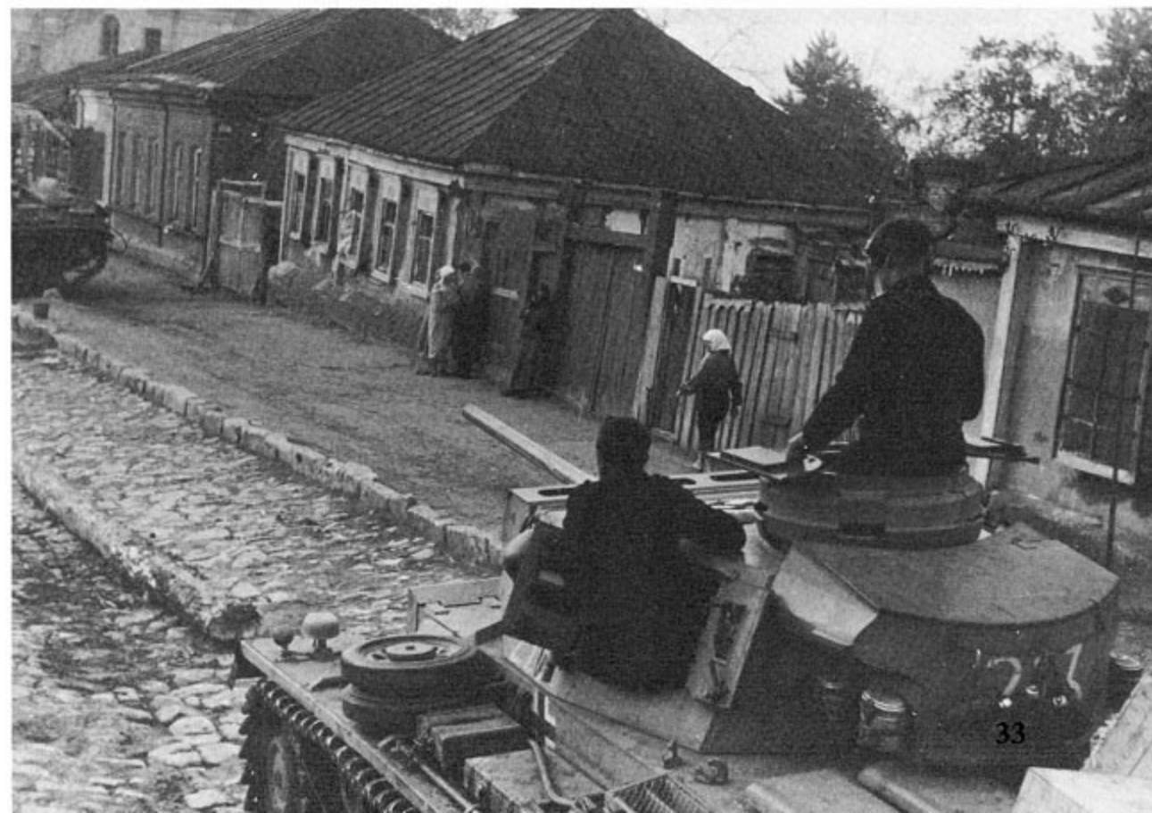
PzKpfw III Ausf Ls drive down a stone street in a Russian village during late 1942. The support frame on the gun mantlet is for spaced 20MM armor which was designed to defeat armor piercing anti-tank rounds. This vehicle is overall Dark Yellow with White turret numbers.
