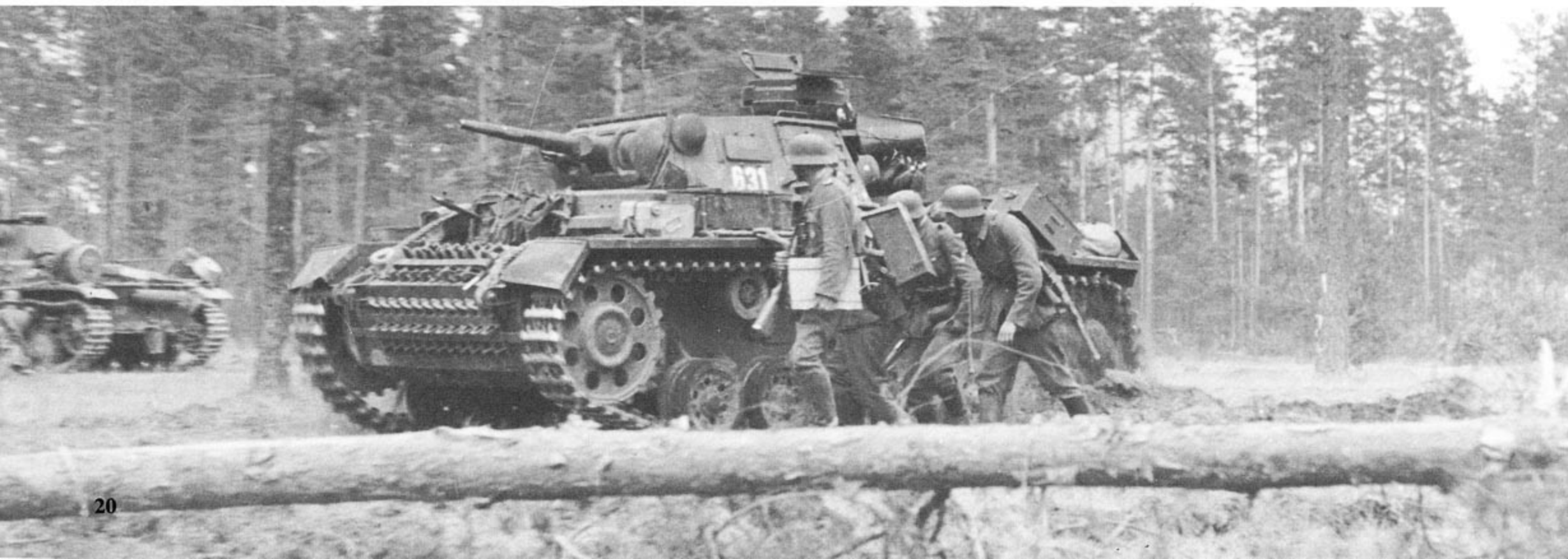
(Above) A pair of PzKpfw III wading tanks during training in preparation for the invasion of Russia. The extended rear exhaust pipes were later adopted for use on the PzKpfw III Ausf M as standard equipment.
