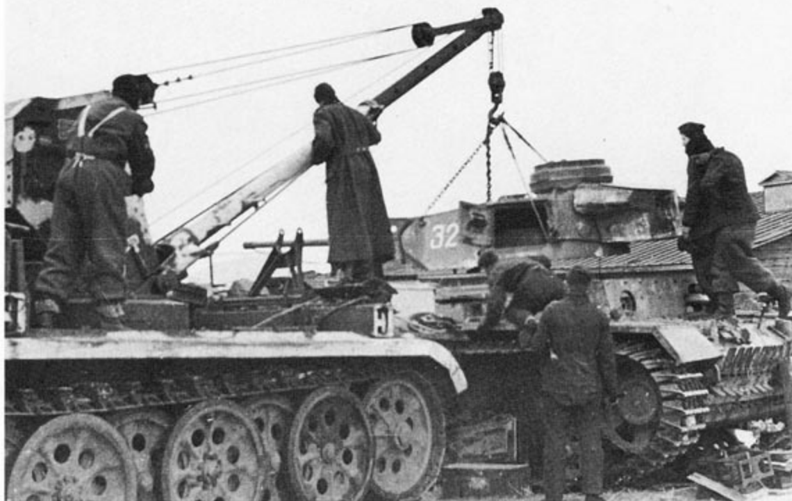
German maintenance crews use a mobile crane to lift the turret off a PzKpfw III Ausf L at a forward repair depot in Russia. The turret basket was removed before the turret was taken off. Because of its bolted-together sub-assemblies, the PzKpfw III could be easily repaired in the field.
