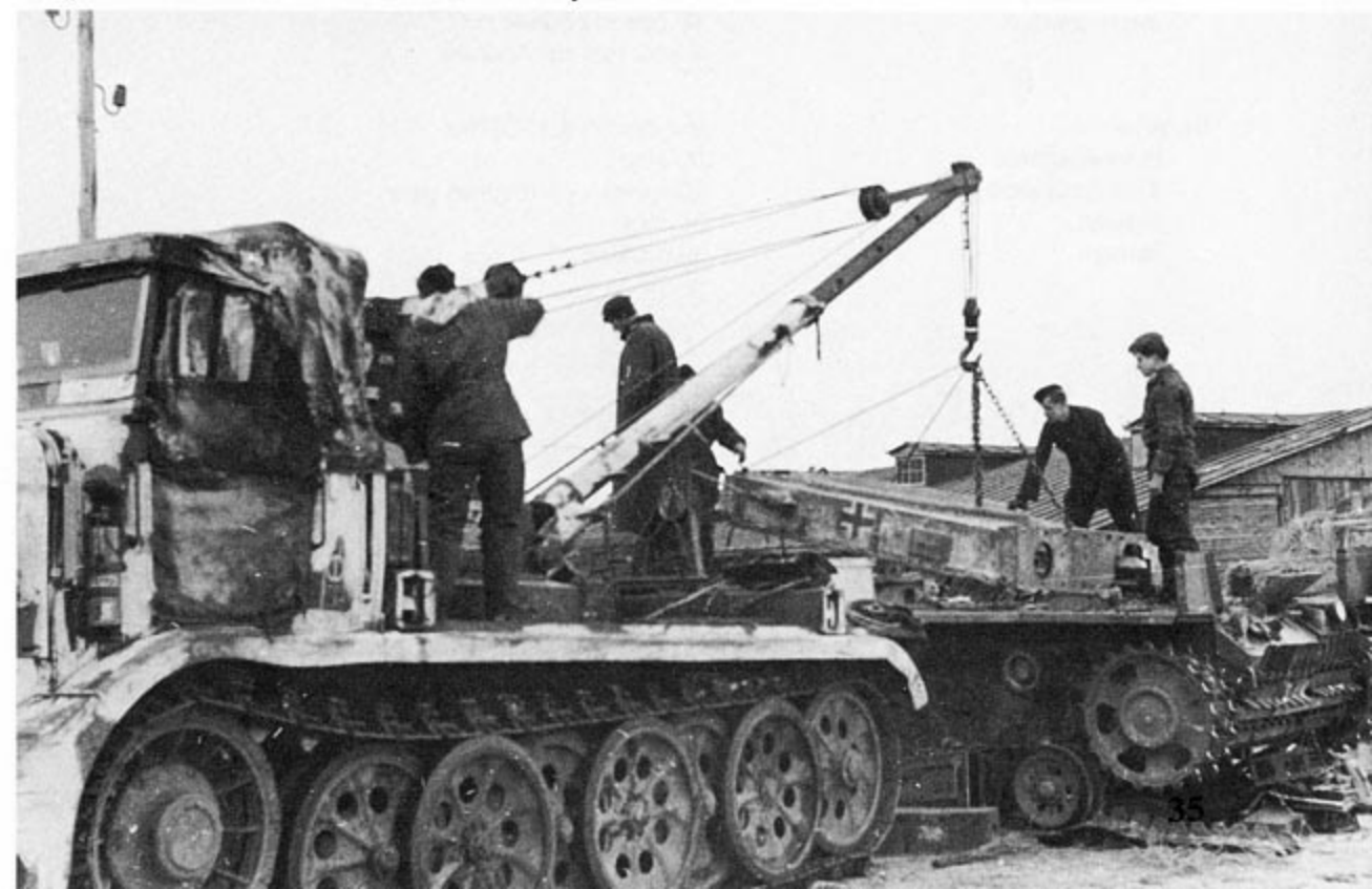
After removing the turret, the superstructure could be easily unbolted from the hull and lifted off. With the superstructure removed maintenance crews could easily reach the transmission, drive train and final drive units for repair or overhaul.
