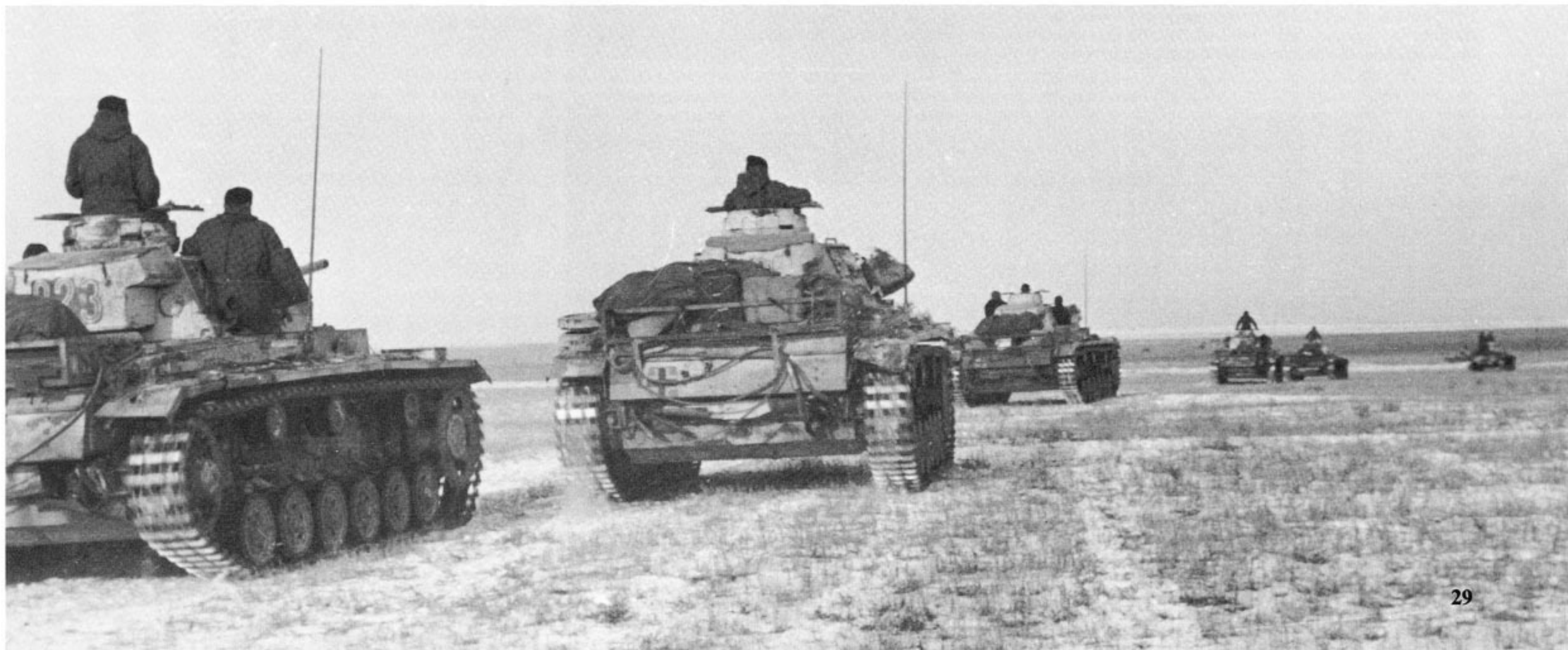
This snow camouflaged PzKpfw III Ausf J has the port vision flap on the mantlet open and has dust covers on all the weapons. The White temporary camouflage was washable and quickly wore off in action.
