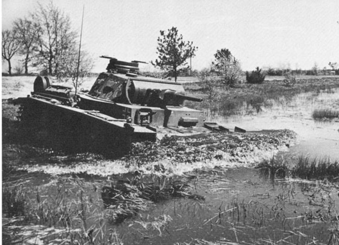
PzKpfw III wading tanks could ford water up to 3 feet deep without special preparations because of the extended rear engine exhaust stacks. This early production PzKpfw III Ausf G wading tank has an early style cupola.
