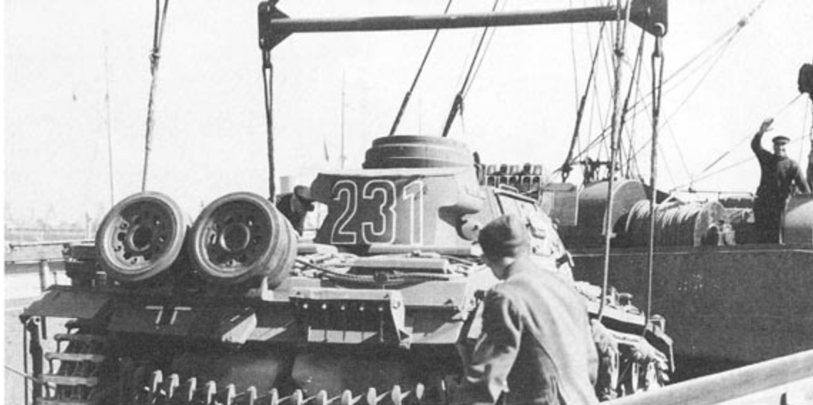
An overall Dark Gray PzKpfw III Ausf G of PzRgt 5, 5.LtDiv, Deutsches Afrikakorps (DAK) is off loaded in Tripoli harbor. The turret number is Red outlined in White. The air vent covers on the engine access hatches were developed for the tropicalized tanks used by the DAK in Africa.
