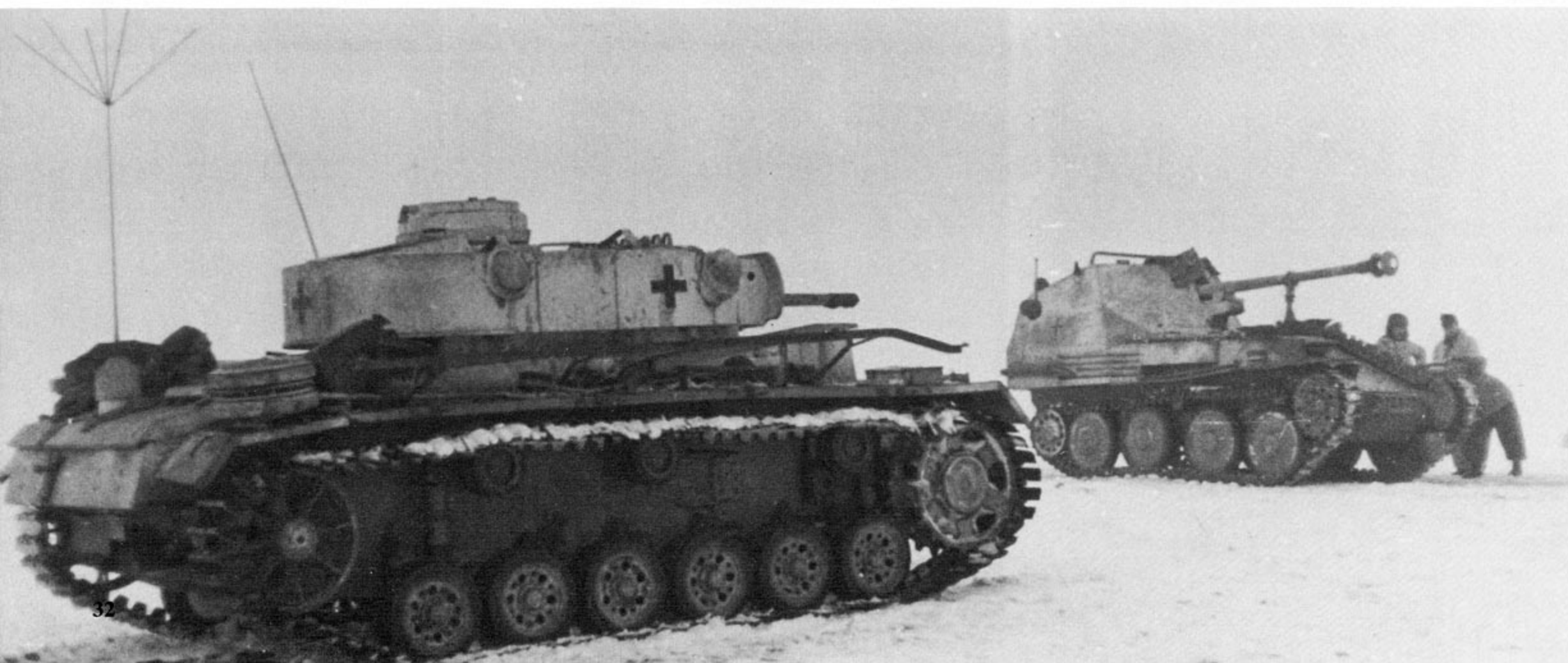
This PzKpfw III Ausf J, believed to be of 1.PzDiv is fitted with a non-standard turret stowage bin similar to those seen on earlier PzKpfw III Ausf Hs. The Dark Gray camouflage has been overpainted with a hand brushed pattern of Dark Yellow.
