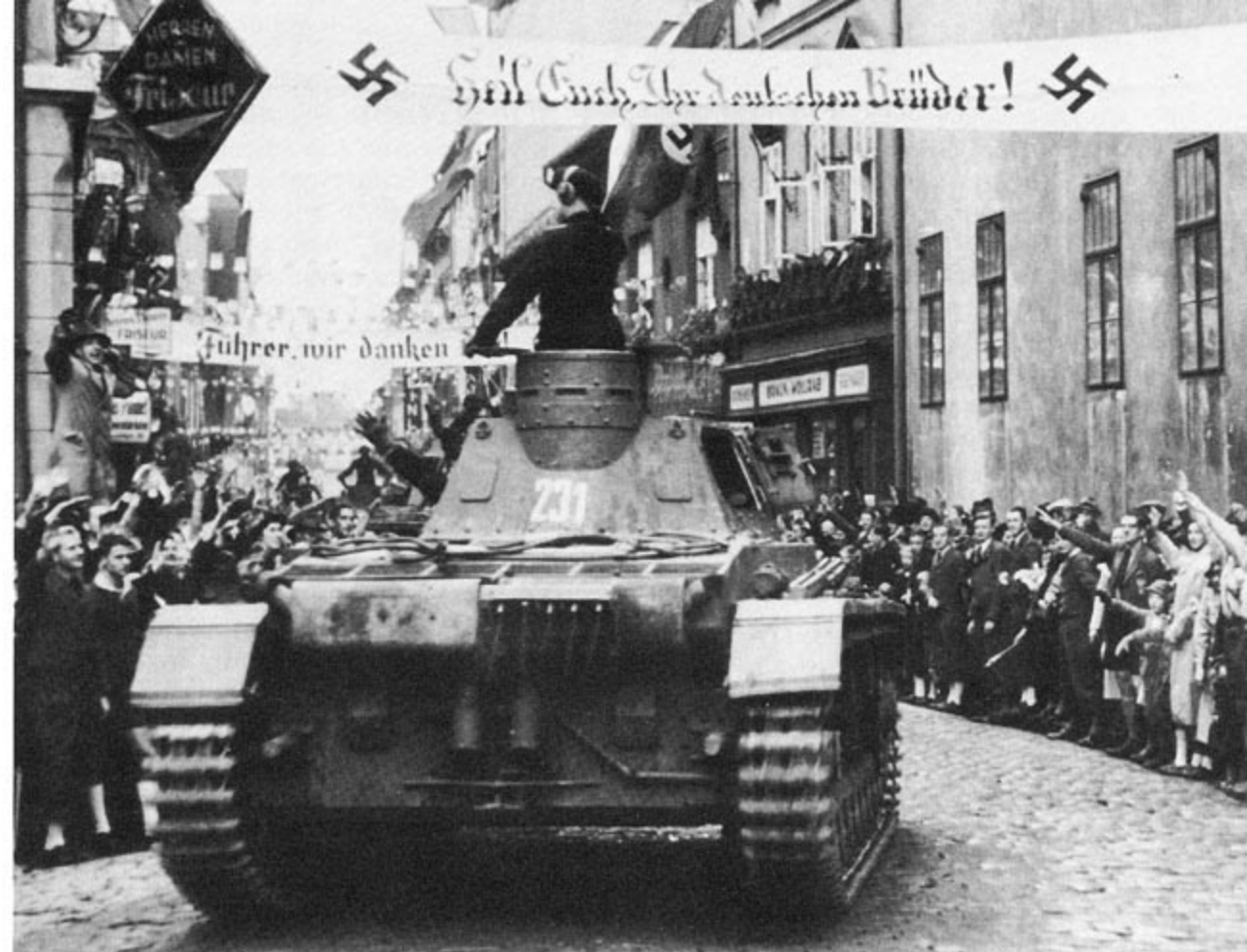
A Panzer III Ausf B enters an Austrian city to the cheers of the populace during the 1938 German occupation of Austria. The smoke candles mounted on the starboard muffler would become a standard feature on subsequent PzKpfw III variants.
