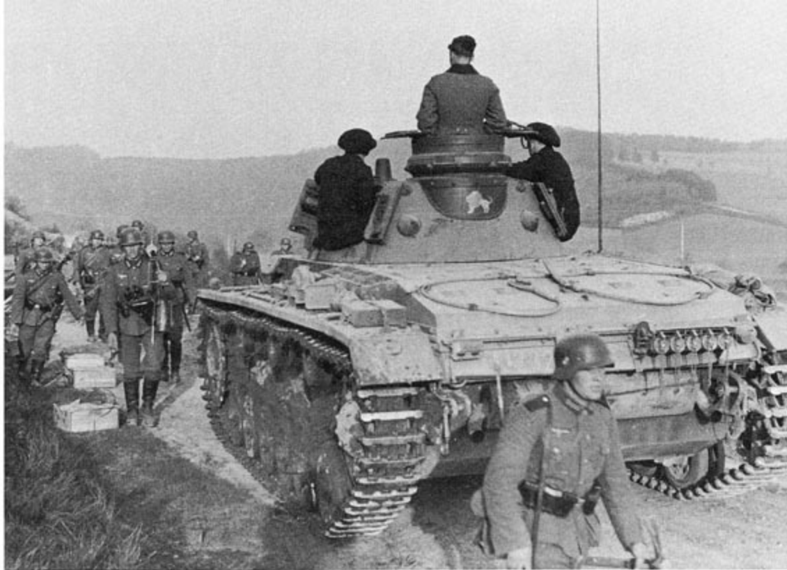
A very dusty overall Dark Gray PzKpfw III Ausf E or F passes infantrymen on a road in the Balkans during 1941. The signal light cover over the left turret roof signal port is in place, however, during maintenance this cover was often removed. A heavy coat of dust has nearly obscured the tank's markings, except for the lion painted on the cupola.
