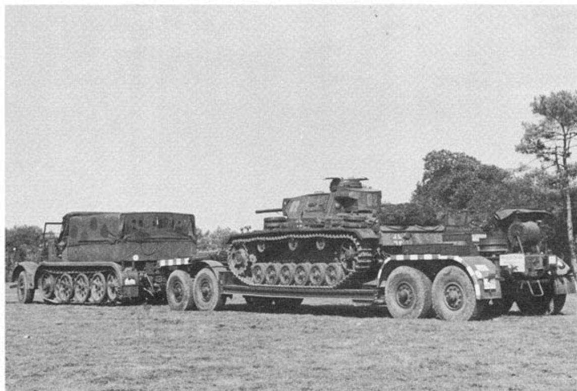
The SdKfz 9 eighteen ton tractor and tank transporter trailer were widely used to carry vehicles between the front and maintenance facilities. The PzKpfw III Ausf L of PzDiv Hermann Goering is painted in a Dark Yellow pattern over a Dark Gray base, with the turret numbers in Red outlined in White.
