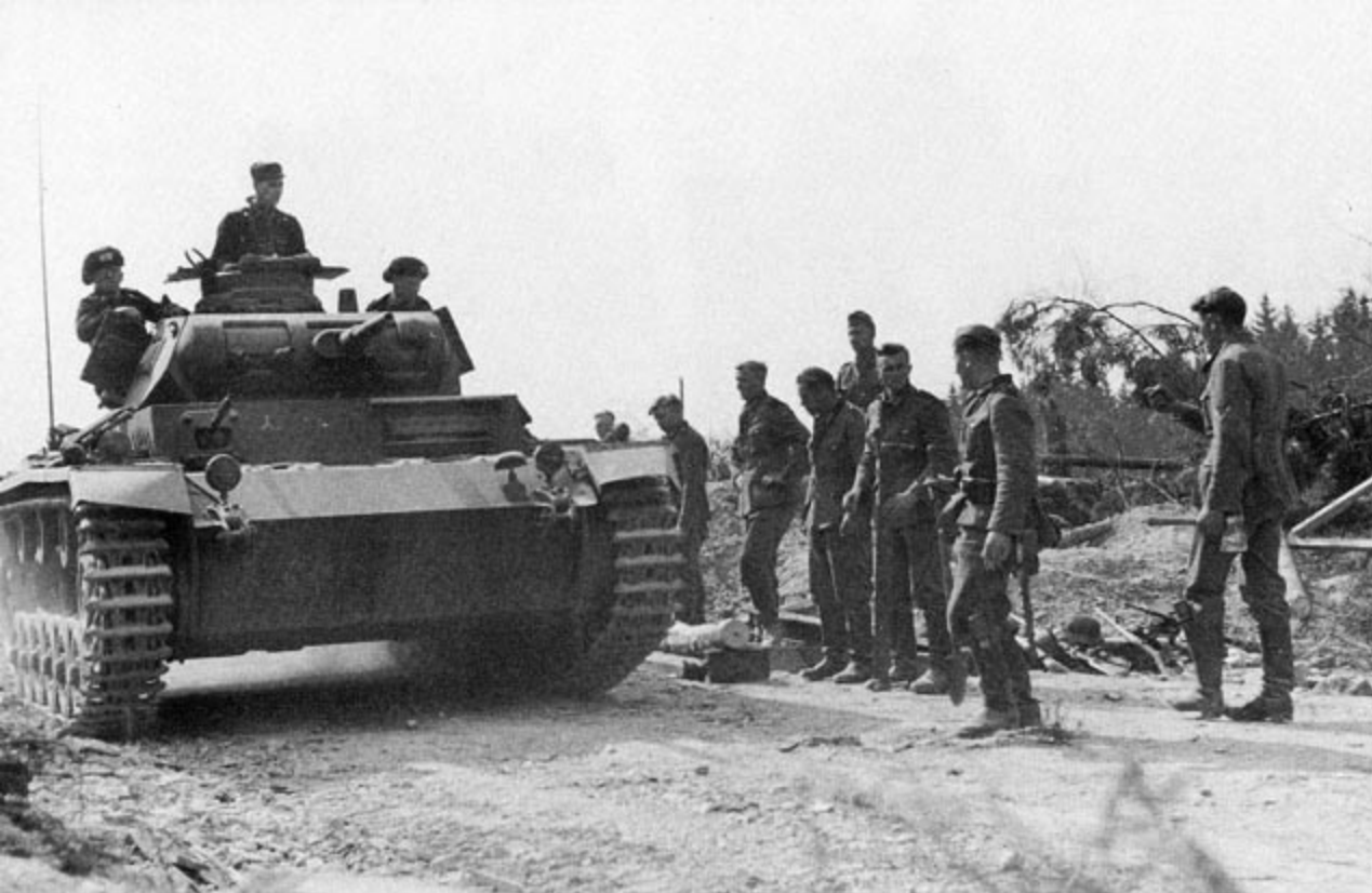
A PzKpfw III Ausf E of 5.PzDiv rolls past a group of infantrymen during the invasion of the Low Countries. The tank is overall Dark Gray with the division sign in Yellow Ochre. The Notek blackout driving light has been moved from its usual position on the port mudguard to the front of the glacis next to the port headlight.
