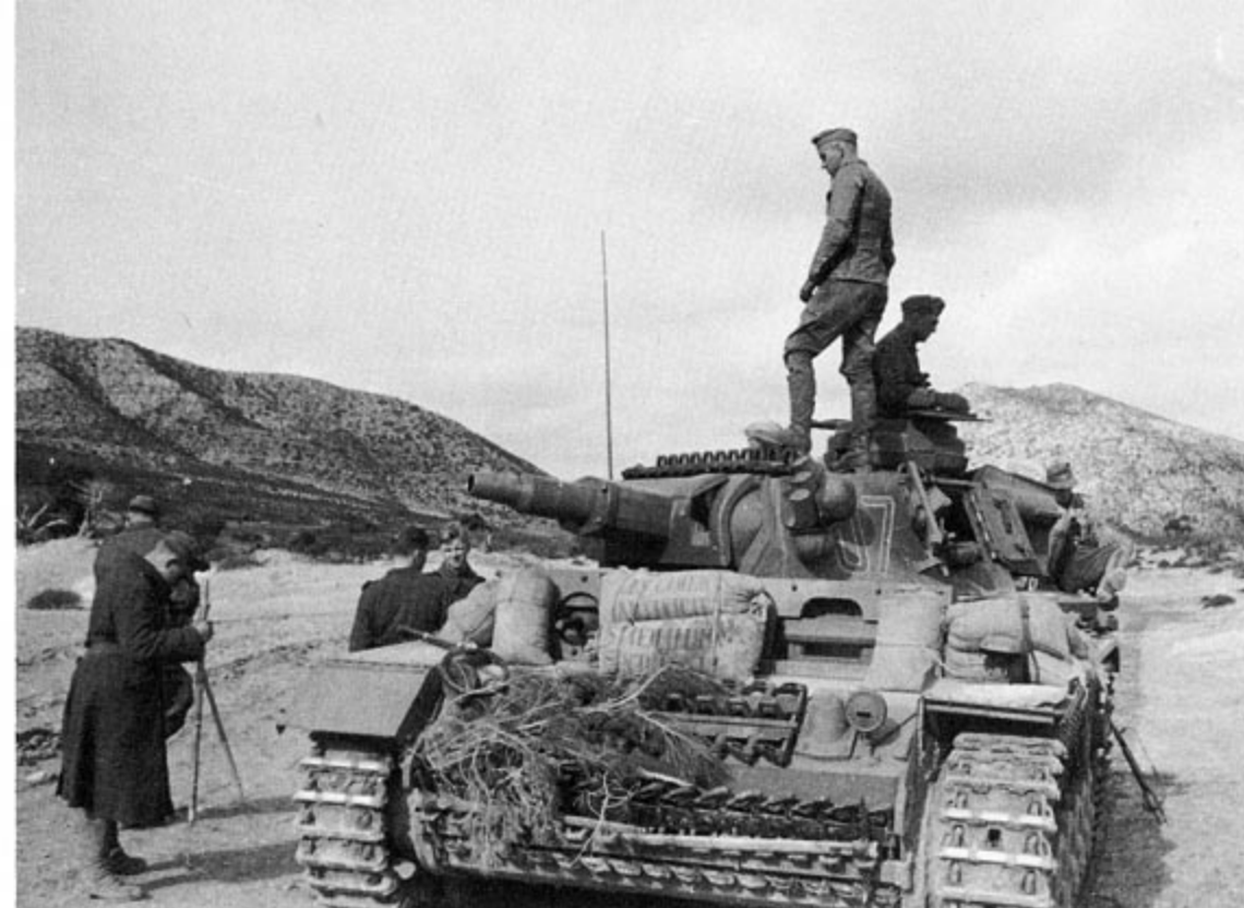
PzKpfw III Ausf N support tanks were used to protect Tiger tanks from enemy infantry and anti-tank units. The sand bags on the front plate are carried for protection against shaped-charge weapons, such as the American bazooka rocket launcher. The turret numbers '07' are in Red outlined in White.
