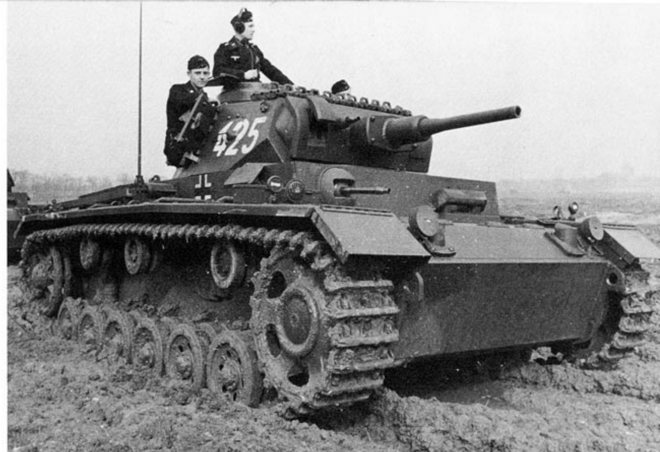
A PzKpfw III Ausf J ploughs through a muddy field during maneuvers in Germany. The revised driver's visor and hull machine gun mount were used on both the PzKpfw III and IV. The Ausf J featured revised glacis hatches, air intake covers, and towing eyes.
