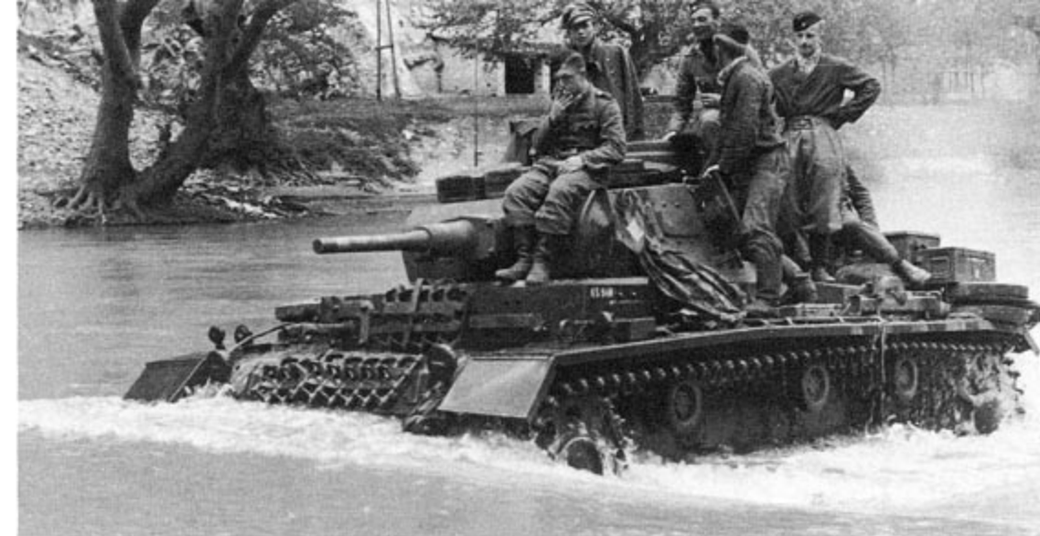
A PzKpfw III Ausf G fords a stream in Greece during late 1941. The chassis number "65940" on the superstructure side indicates that this was one of the last Ausf G's built. The overall Dark Gray camouflage is broken only by the White chassis number, diamond playing card symbol, and the Yellow Ochre 2.PzDiv sign on the superstructure plate.
