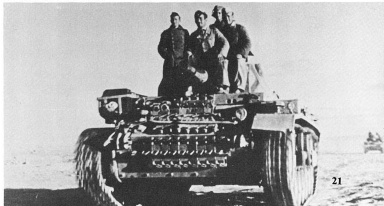
A PzKpfw III Ausf H of PzRgt 5, 21.PzDiv (formerly 5.LtDiv) advances across the desert near Marmarika, Libya in December of 1941. PzRgt 5 equipped most of its vehicles with external stowage racks for fuel and water jerry cans. The extra track links on the hull and superstructure front were for added protection against armor piercing anti-tank rounds.
