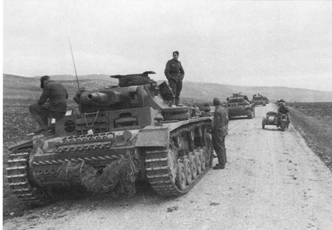
PzKpfw III Ausf N support tanks of sPzAbt 501 wait along side a road in Tunisia during late 1942. The Ausf N (based on the Ausf L chassis) has been fitted with a gun travel lock mounted on the superstructure decking. This vehicle is overall desert Brown, covered with a thick layer of dust with the turret numbers '113' in Red outlined in White.
