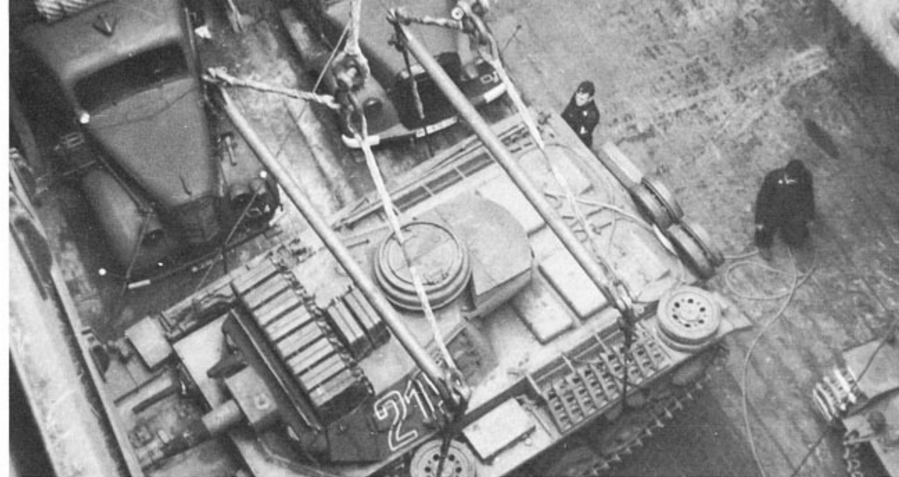
(Above) A tropicalized PzKpfw III Ausf G is lowered to the dock after being off loaded from a German freighter in Tripoli. The stowage racks for carrying water filled jerrycans were fitted to tanks of PzRgt 5 for operations in the desert.
