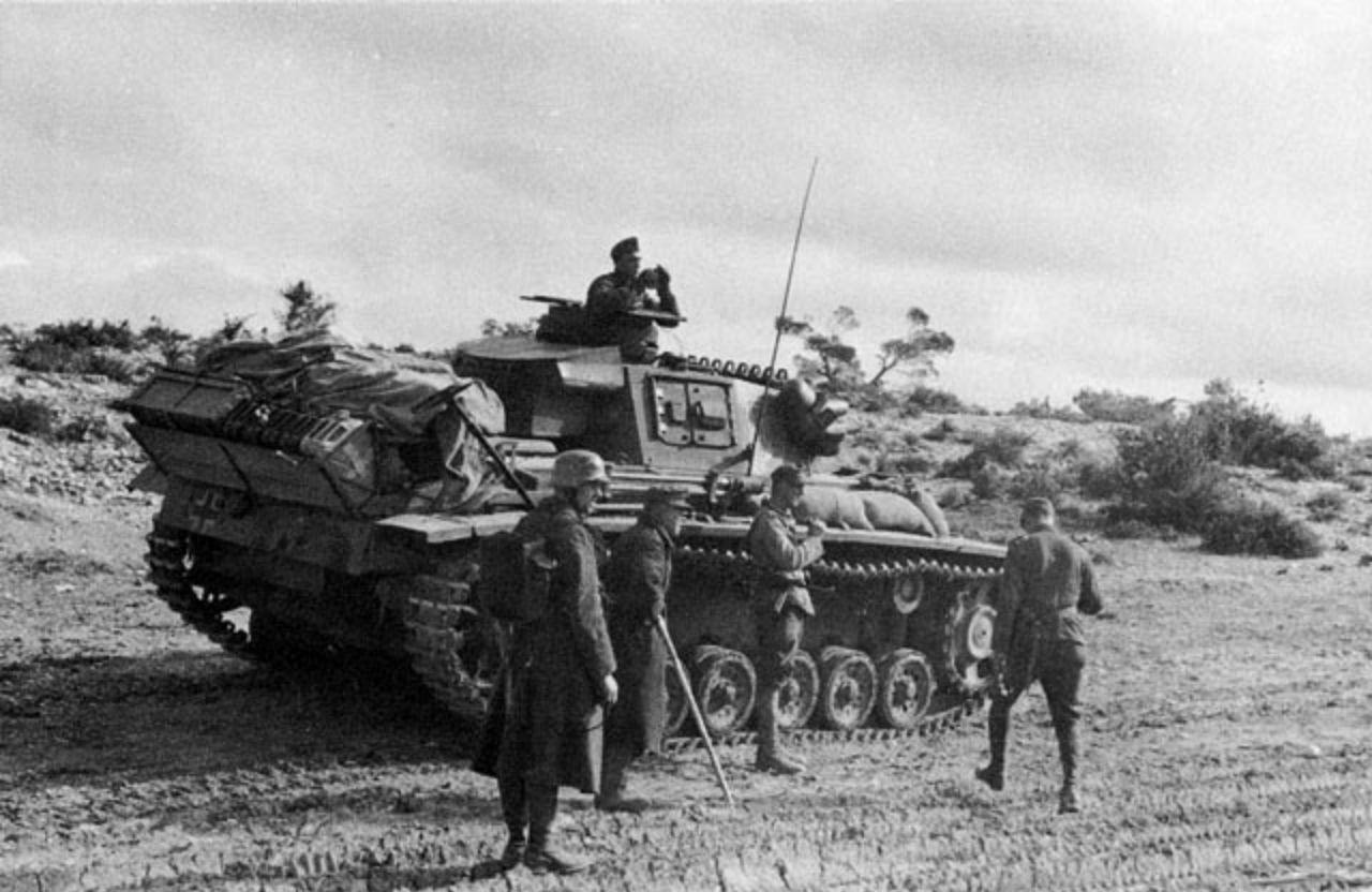
A PzKpfw III Ausf N support tank of sPzAbt 501 waits alongside a Tunisian road for the word that the way is clear of mines. The jerry cans carried on the field installed stowage rack on the rear deck are for water not fuel.
