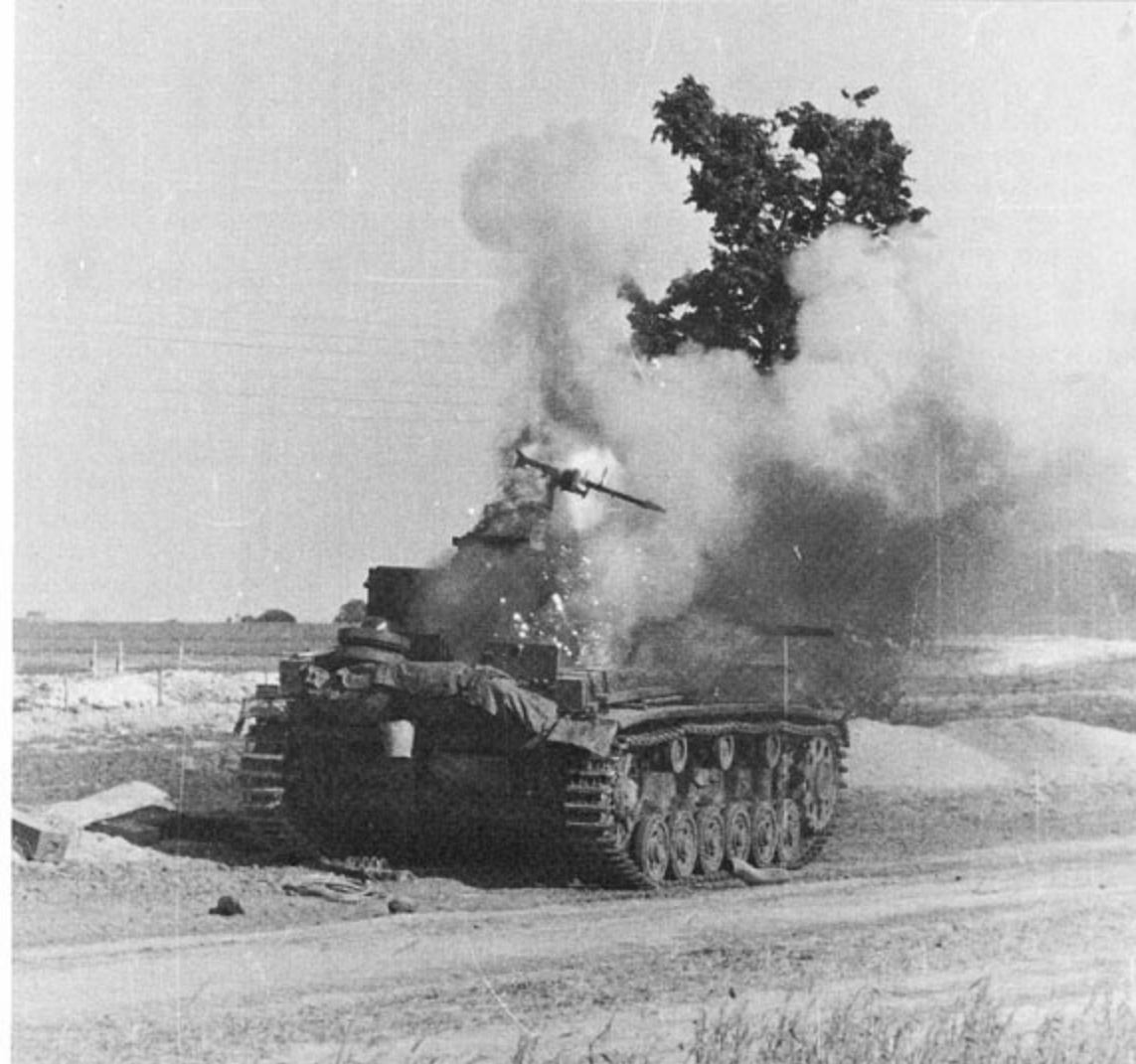
A PzKpfw III Ausf H, hit on a Russian road during June of 1942, has been set afire and its ammunition is cooking off. The chassis is the early production version with the 360mm track and early style drive sprocket, idler wheel, and return roller locations.
