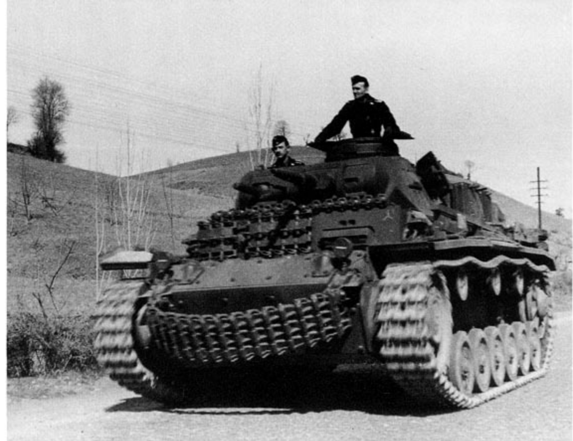
An overall Dark Gray PzBefWg III Ausf H of 2.PzDiv advances down a Greek road at high speed. This vehicle carries bolted-on armor plate on the glacis and hull front plate along with spare track links on the superstructure front, top, and hull front plate.
