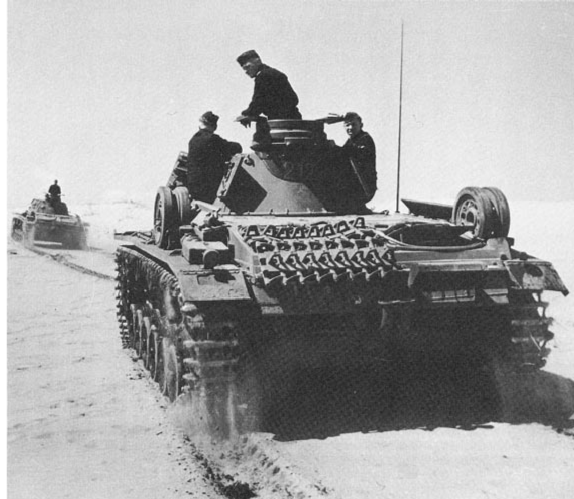
(Above) A pair of PzKpfw III wading tanks during training in preparation for the invasion of Russia. The extended rear exhaust pipes were later adopted for use on the PzKpfw III Ausf M as standard equipment.
