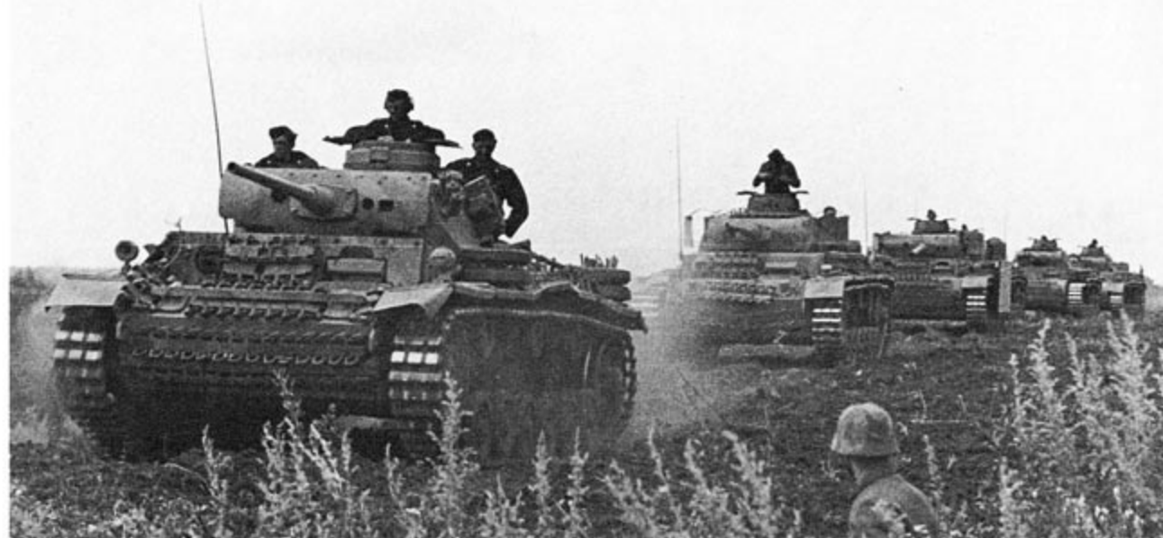
A column of PzKpfw III Ausf M tanks move up past infantry positions during the Don campaign in southern Russia. The first and third vehicles are Ausf Ms while the second tank is an Ausf J. The lead tank is fitted with turret smoke dischargers, spaced armor, and Bosch blackout headlights mounted on the fenders.
