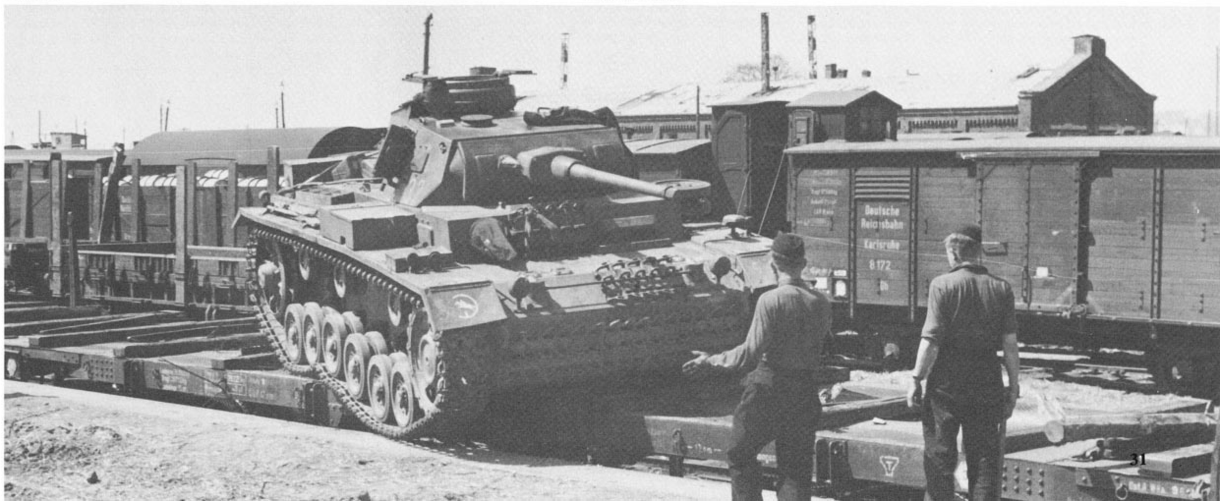
Crewmen of 24.PzDiv ease a PzKpfw III Ausf J off a flatcar prior to beginning the Stalingrad campaign. The vehicle is overall dusty Dark Gray, with the 1.Cavalry Division sign in White on the starboard fender. This vehicle is armed with the L/60 gun and has stowage boxes fitted on the fenders.
