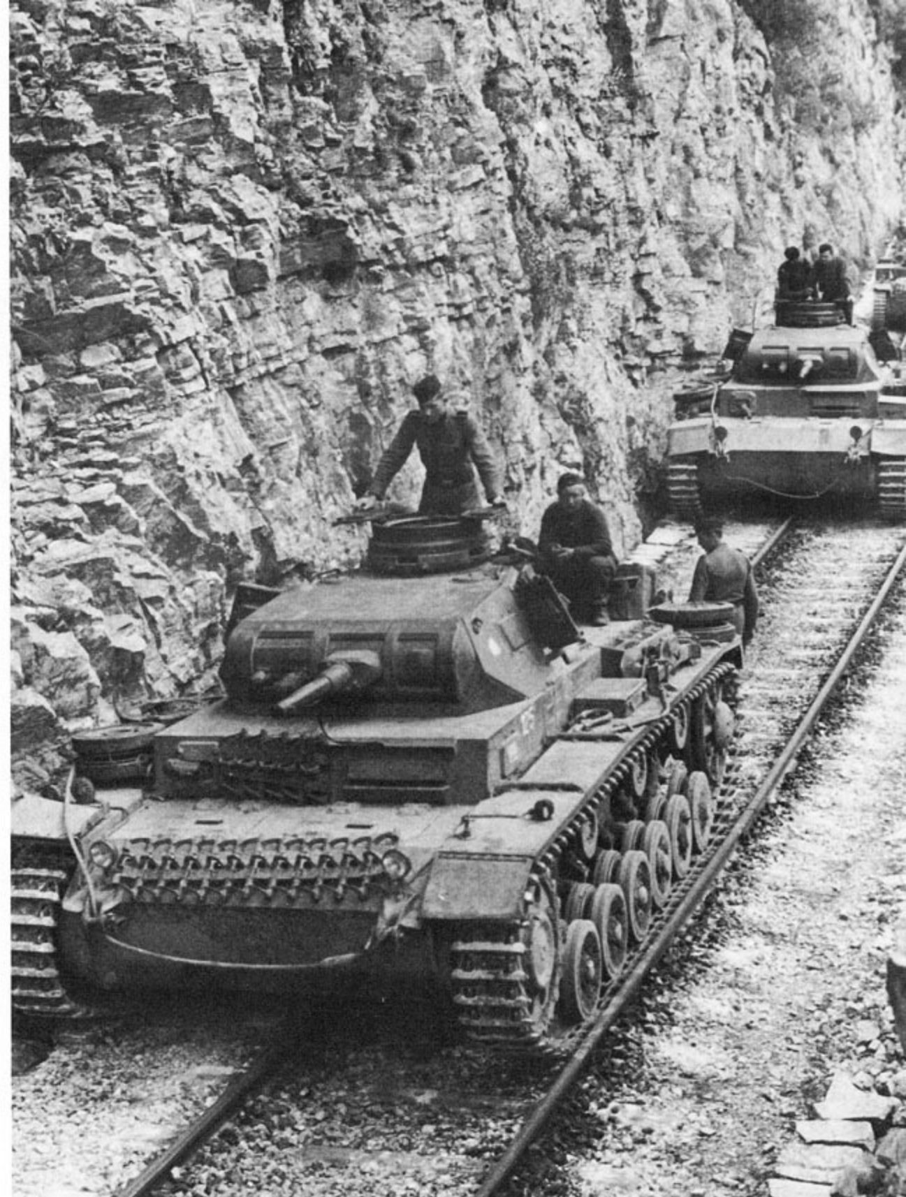
A column of PzKpfw III Ausf Es of 2.PzDiv advances along a railway in the Greek mountains during the 1941 invasion of Greece. The dusty overall Dark Gray camouflage blended well in this rocky country. The lead vehicle has dust covers fitted over the two turret co-axial machine guns.
