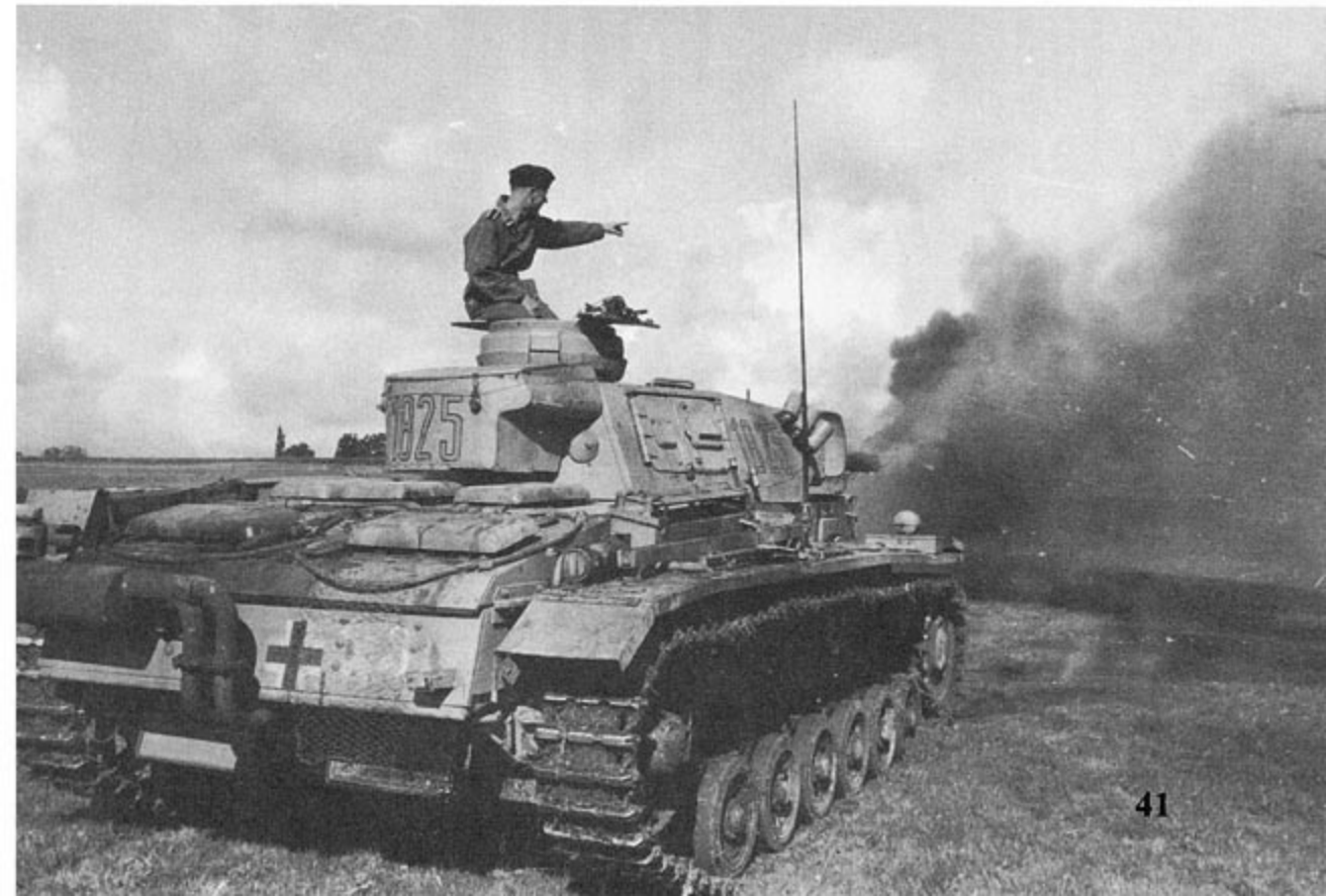
The Flammenwerfer-Panzer III Ausf M carried the same wading gear fitted to gun armed Ausf Ms. The high muffler is at the far left and the side air intakes are fitted with sealing flaps and their retainer frames. This tank is overall Dark Yellow, with Yellow Ochre numbers outlined in Black.
