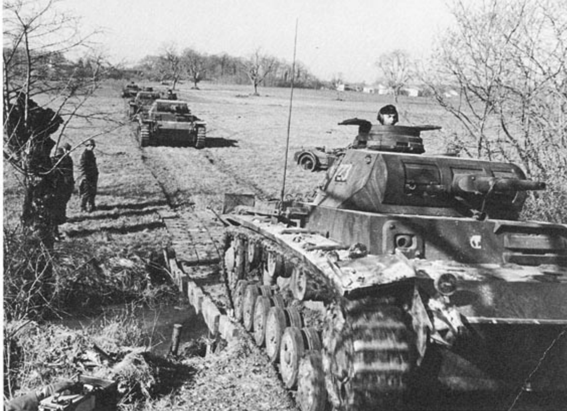
Overall Dark Gray PzKpfw III Ausf Es cross a temporary field bridge in France. The internal mantlet has two armored sleeves for the co-axial MG 34 machine guns on the starboard side of the main gun. The radio mast was hinged and could be folded down into the metal tray on the starboard side of the hull.
