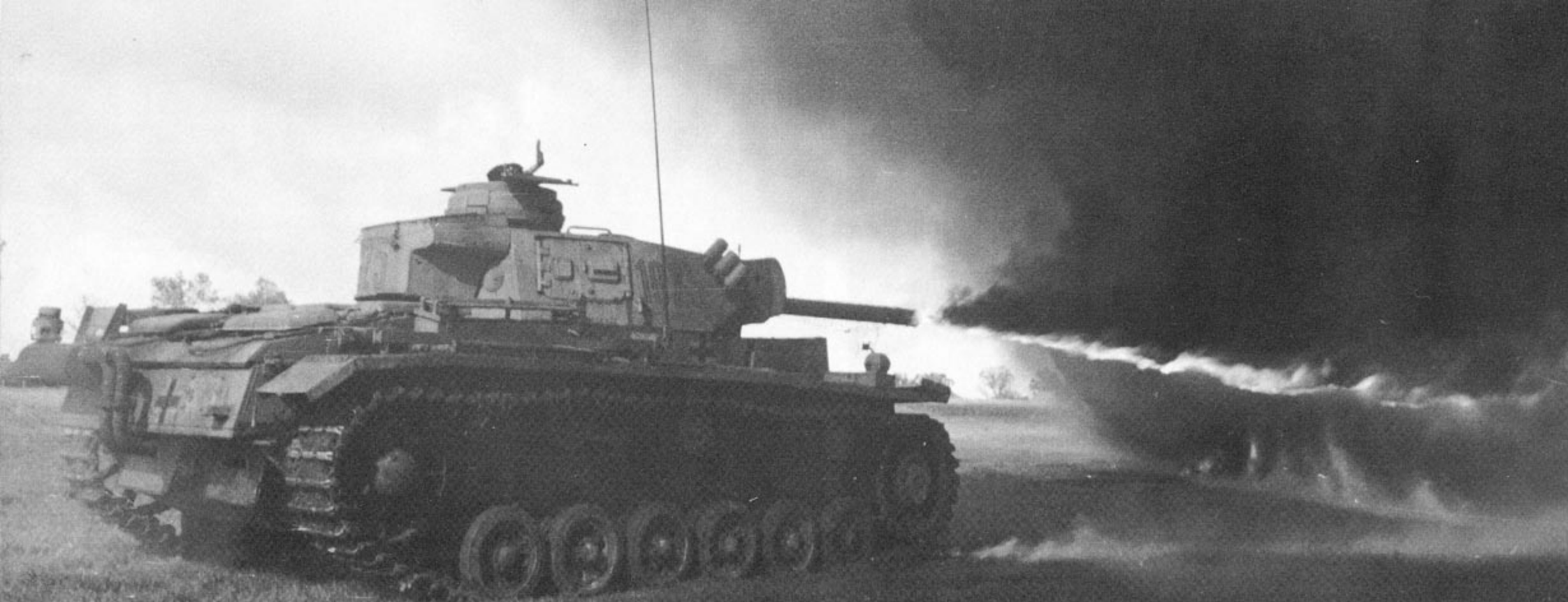
(Above) A PzKpfw III Ausf M (FI) fires its main weapon, a flame projector with an effective range of 180-197 feet. The flame projector barrel was heavier than the 50mm L/60 gun barrel, but was hard to distinguish from the standard tank gun from a distance.
