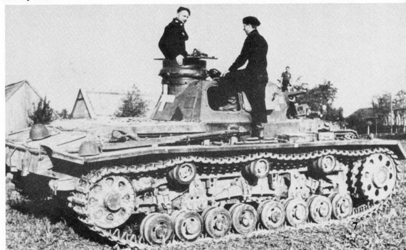
The crew of a PzKpfw III Ausf D relaxes for a moment during the 1939 invasion of Poland. The multiple leaf suspension, cast turret cupola, and extended rear upper tailplate were features of the Ausf D. The early chassis designs of the PzKpfw III were complicated and vulnerable to enemy fire.
