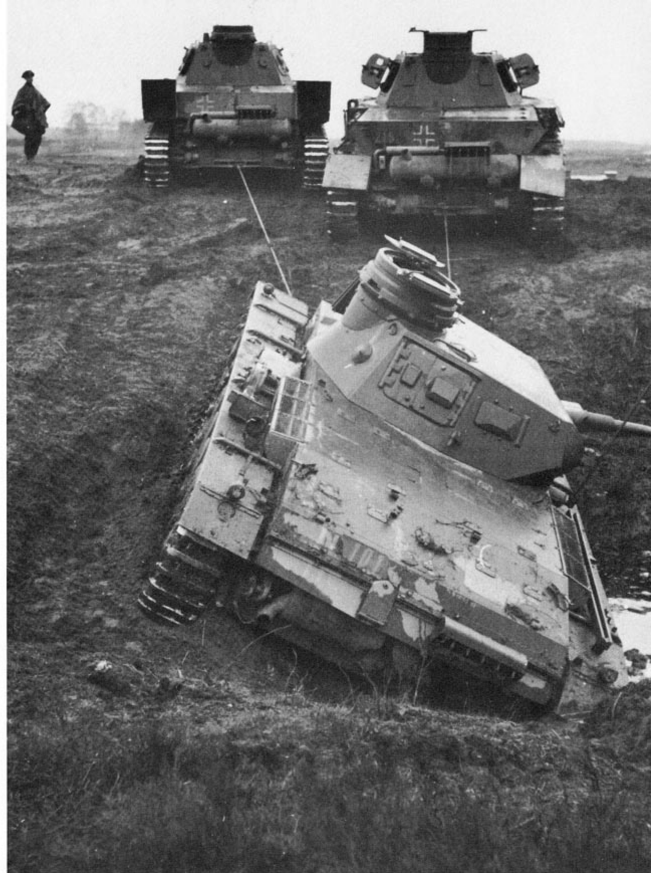
Two PzKpfw IVs attempt to tow a bogged down PzKpfw III Ausf E out of a muddy shell hole. The PzKpfw IV on the left has the rear fender mud guards raised to prevent them from becoming caked with mud thrown up by the tracks and possibly fouling the idler wheel.
