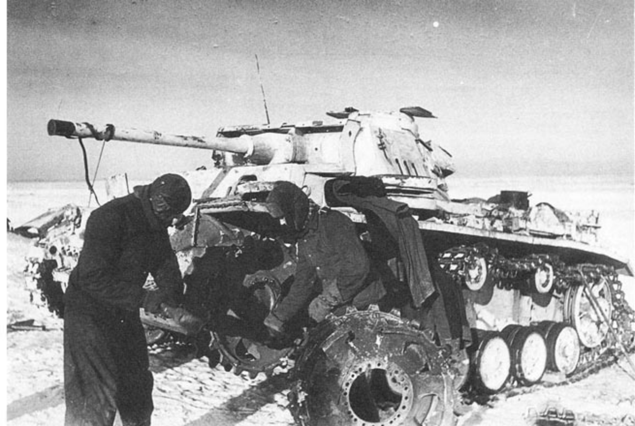
Crewmen work to replace the damaged drive sprocket of a snow camouflaged PzKpfw III Ausf L of 3.PzGrenDiv. The replacement drive sprocket is Dark Gray and the turret numbers and division sign are in Black. The frame on the mantlet is for 20mm spaced armor.
