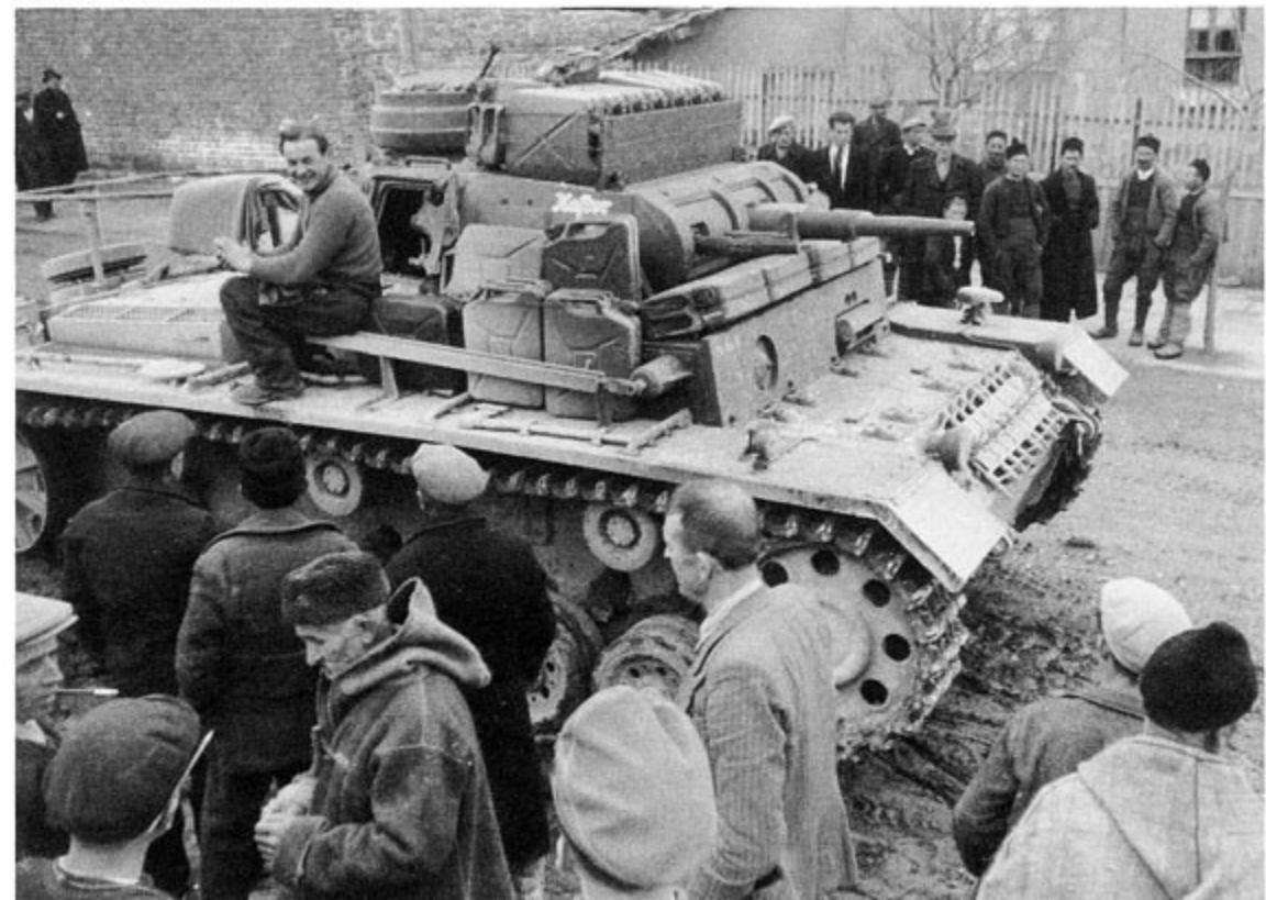
A PzBefWg III Ausf H passes through a Balkan village during 1941. The vehicle is Dark Gray with a heavy layer of dust. The White name Kastor has been painted on the turret side in Old Gothic lettering. 'fu 6u.8' in White on the superstructure front plate identified the type of radio equipment carried.
