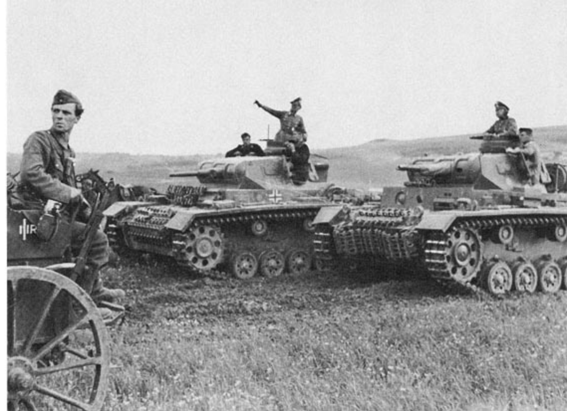
A PzKpfw III Ausf E of 13.PzDiv (background) has pulled alongside a Panzerbefehlswagen III Ausf H (PzBefWg III) on the Russian steppes during OPERATION BARBAROSSA, the 1941 invasion of Russia. The PzBefWg III was a command tank variant of the PzKpfw III fitted with extensive radio equipment.
