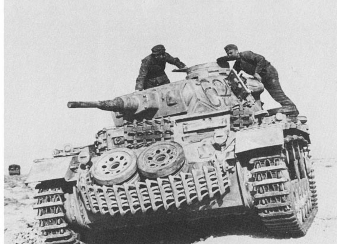
The last 100 PzKpfw III Ausf Fs were up-gunned with the 50mm KwK L/42 cannon during production and the majority of older vehicles were retro-fitted with this weapon during factory overhauls. The roadwheels hung on the extra track on the glacis served as spaced armor to help break up armor-piercing projectiles.
