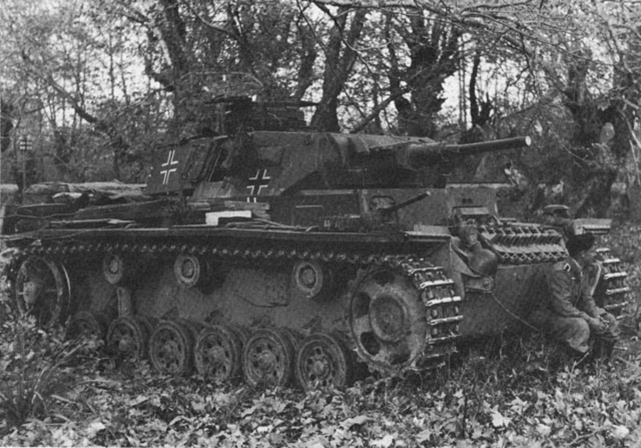
This late production PzKpfw III Ausf H of 1.PzDiv has the revised drive sprocket and rear idler installed for use with the 400mm track. This vehicle has been fitted with a non-standard rectangular turret stowage box which is larger than the standard production box.
