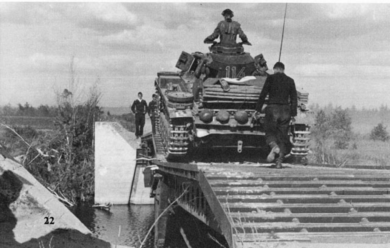
An overall Dark Gray PzKpfw III Ausf H crosses a temporary bridge across a stream in Russia. The turret stowage box is the standard production version with cutaway sides to clear the rear turret pistol ports. The turret numbers are Red outlined in White.
