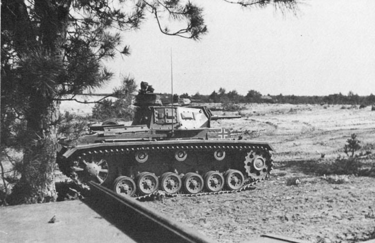
A PzKpfw III Ausf G wading tank with the engine side air intakes raised to improve engine cooling. These waterproof covers could be released from inside the vehicle once it was on dry land. '213' is overall Dark Gray with Yellow Ochre turret numbers. The bear on the turret side is Red with a White border.
