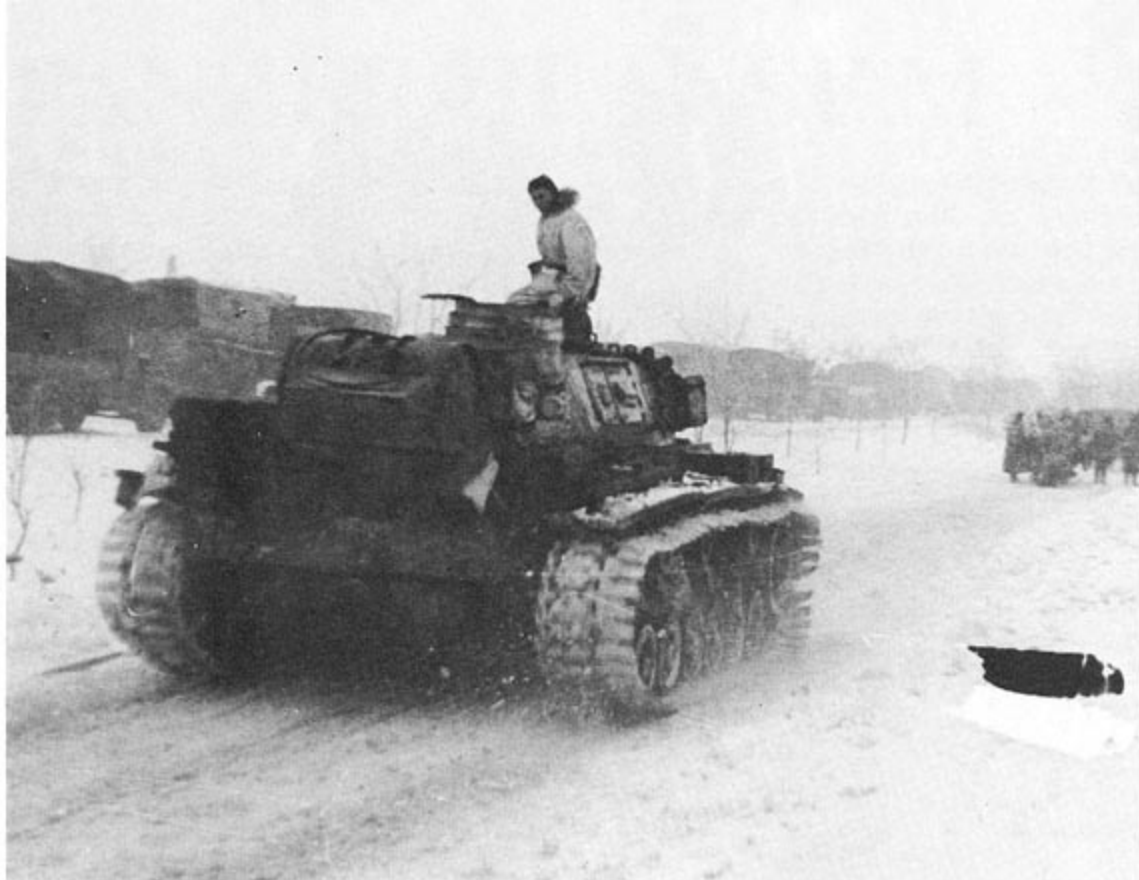
This early production Ausf L is equipped with Ostketten extended tracks. These tracks were easily damaged as is evidenced by the bent and broken track extensions. The badly worn snow camouflage is compromised by the extensive external stowage on the rear deck.
