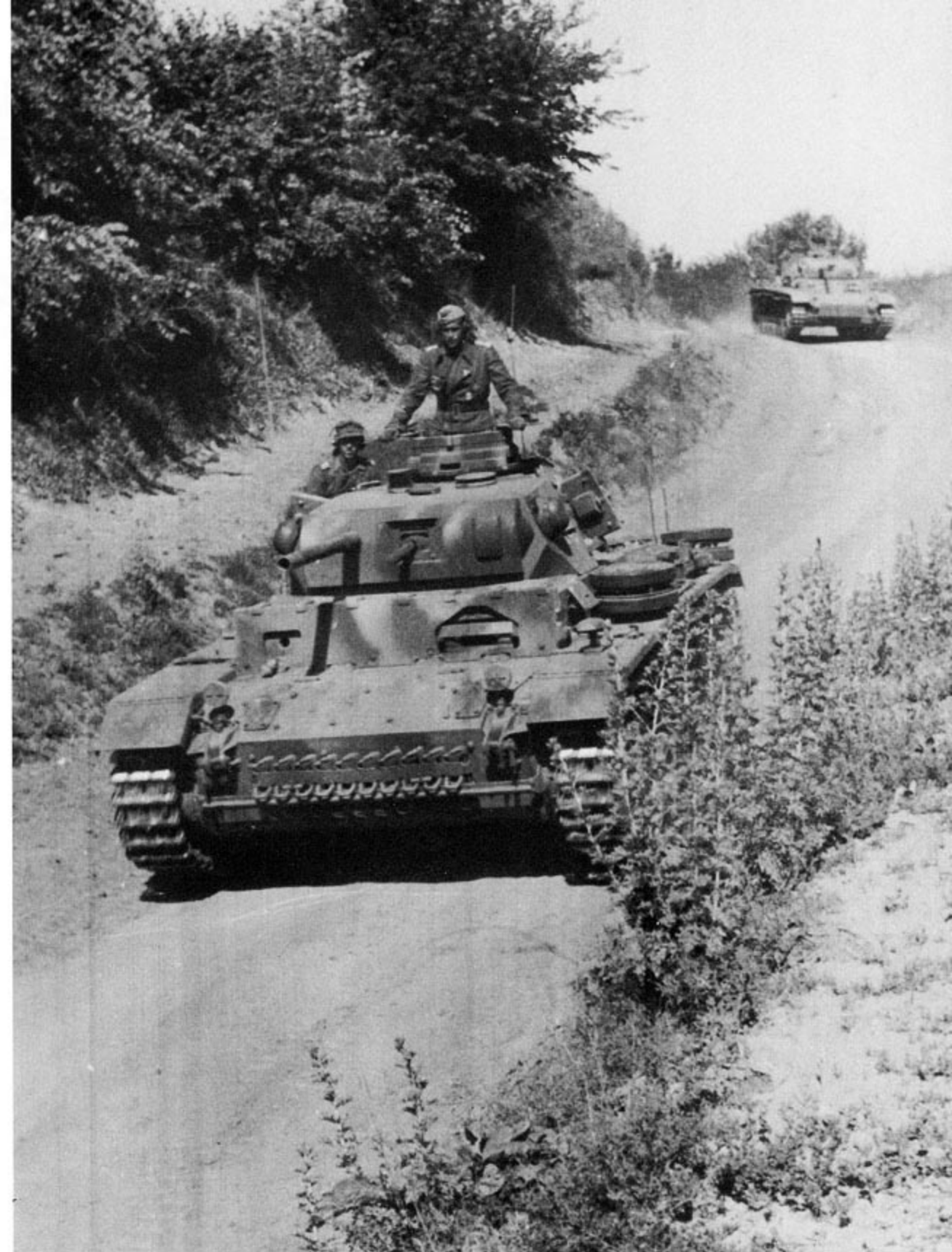
A Panzerbeobachtungswagen III (armored observation vehicle) moves down a dirt road in Russia during 1943. PzBeobWg III Ausf Gs carried extra armor plate on the front and rear of the vehicle, a dummy gun in place of the co-axial MG 34 machine gun and a flexible MG 34 centrally mounted in the mantlet.
