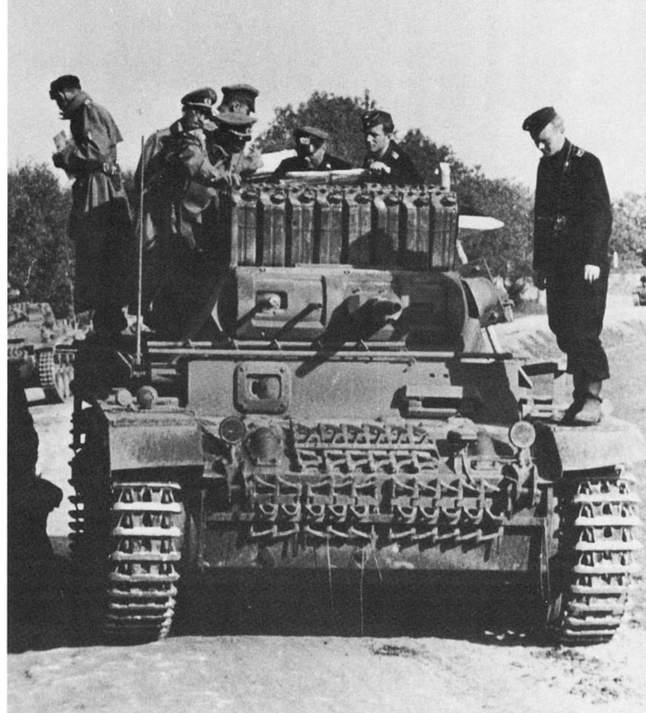
Staff officers hold a conference on the turret roof of a PzBefWg III Ausf E in Russia during early 1941. The jerry cans on the turret roof are for extra water and the extra track sections are secured in place on the hull front with welded bars.
