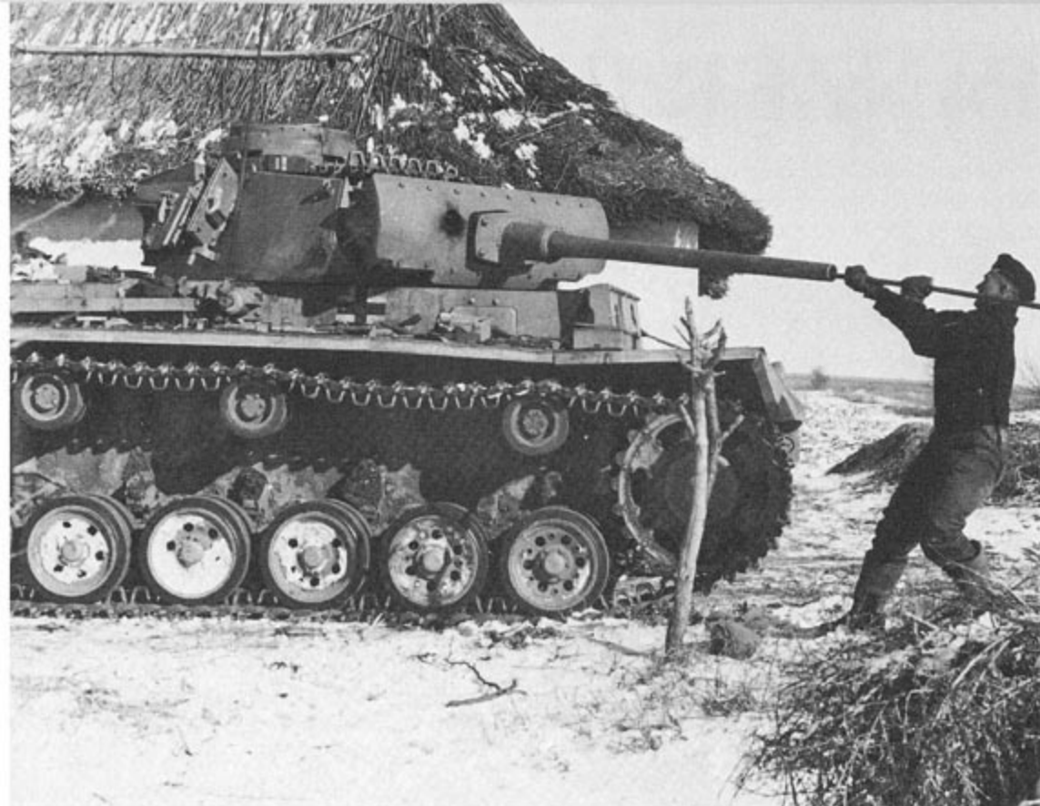
A crewman cleans the long barreled 50mm L/60 gun of a PzKpfw III Ausf L outside a Russian hut during the Spring of 1943. The 20mm spaced armor was bolted to a subframe attached to the mantlet which kept the armor at the proper distance from the mantlet for maximum protection.
