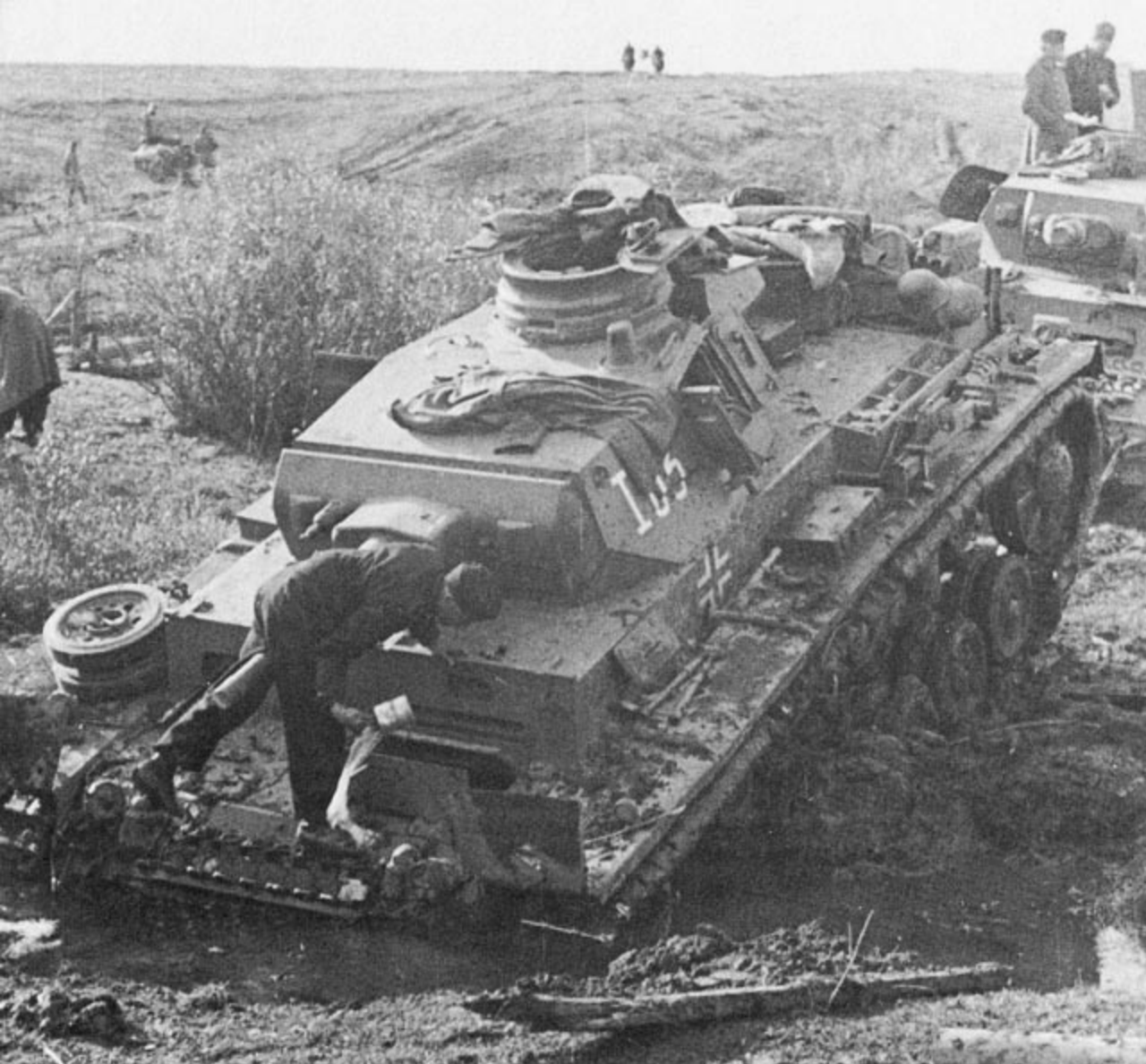
A crewman bails water out of a PzKpfw III Ausf F of 1.PzDiv that has become mired in a Russian stream. The tank is armed with the 50mm KwK L/42 gun in an external mantlet and has 30mm armor plate added to both the hull and superstructure front.
