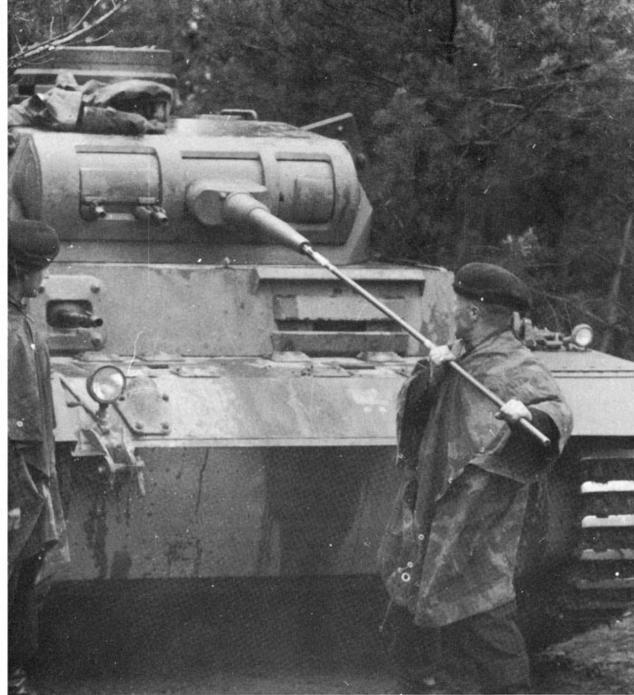
A crewman cleans the 37mm main gun of a PzKpfw III Ausf F of 2.PzDiv. The Ausf F can be distinguished from the nearly identical Ausf E by the armored covers over the drive unit air intakes on the glacis (one of these covers is next to the starboard headlight).
