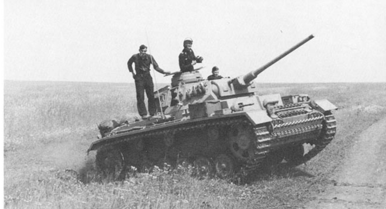
An overall Dark Yellow PzKpfw III Ausf J crosses an open field in Russia during 1941/42. The small turret number '322', partially obscured by water bottles strung on the turret side, is in Black. The long barreled L/60 gun increased the overall length of the vehicle by 2.46 feet.
