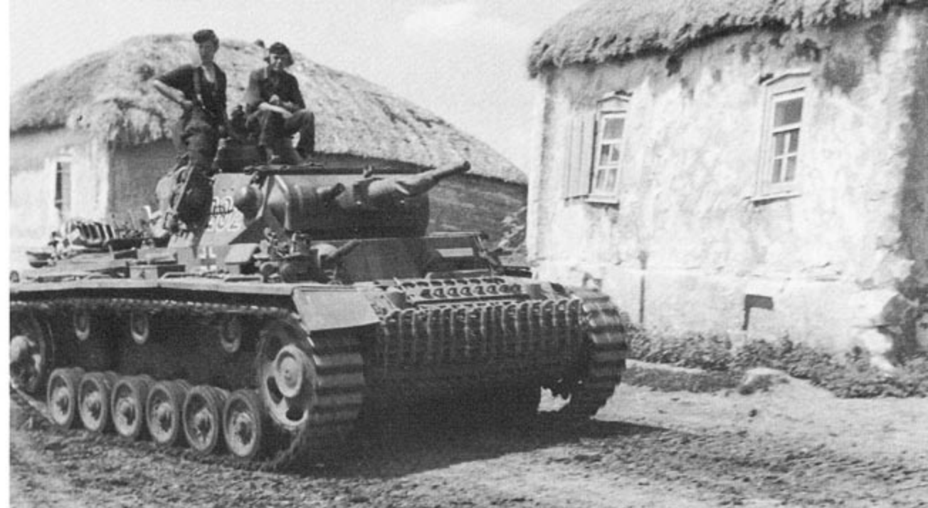
A PzKpfw III Ausf J of 23.PzDiv passes through a Russian village behind the lines. Dust covers have been installed on all the tank's guns to protect them from dirt and dust. The crew has added two layers of spare track to the hull front for extra protection from anti-tank rounds.
