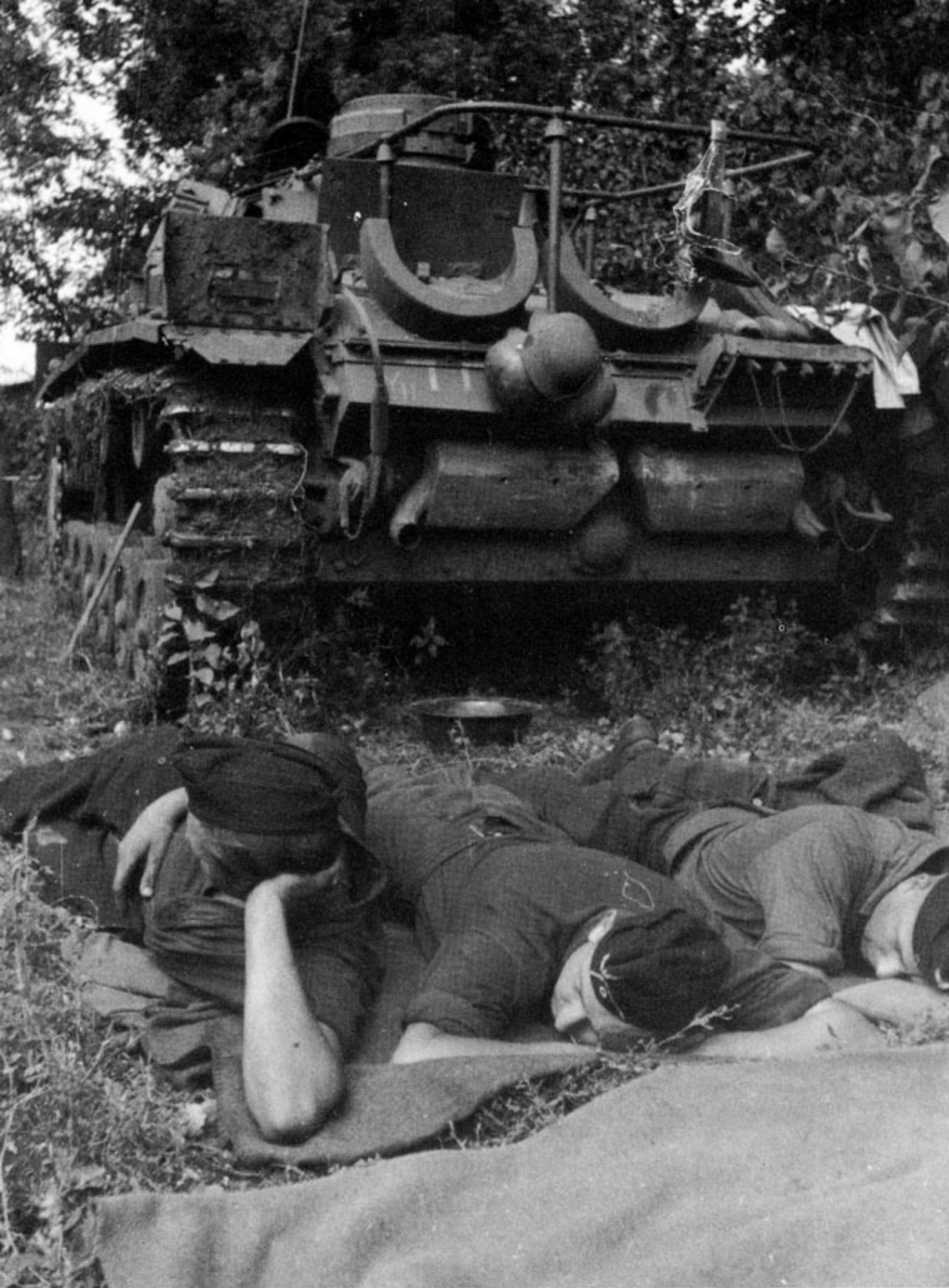
The crew of this PzBefWg III Ausf H of 9.PzDiv takes advantage of a quiet moment on the Russian Front to get some sleep. The semi-circle mounts on the engine deck rear are spare road wheel stowage brackets. The vehicle is overall Dark Gray with a Yellow Ochre division sign on the port side of the rear plate.
