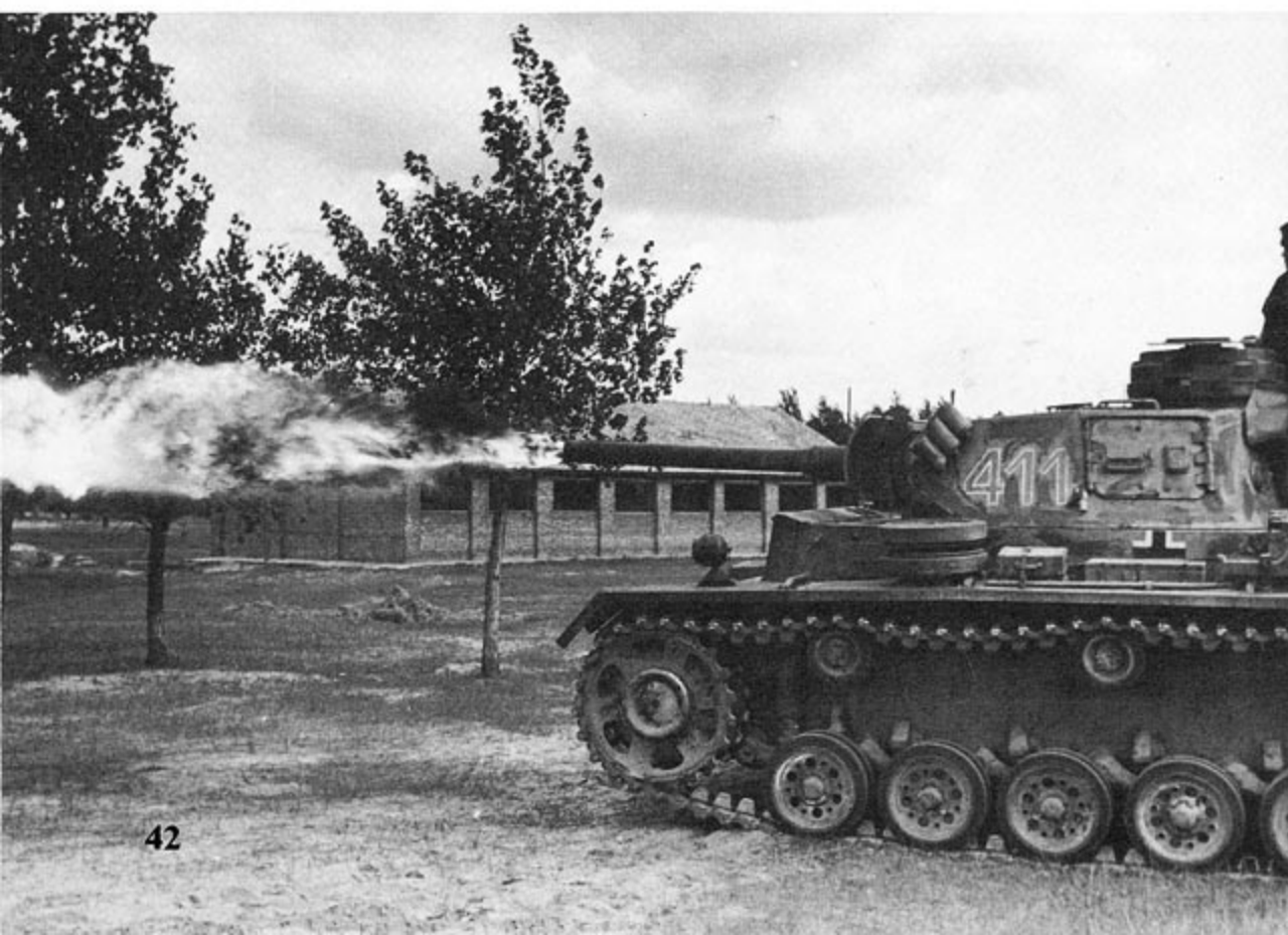
(Below) A Flammenwerfer-Panzer Ausf M tests its main armament before going into action. The flame projector was very effective against pill boxes and other fortifications, but the vehicle had to get in close in order to bring the weapon within effective range.
