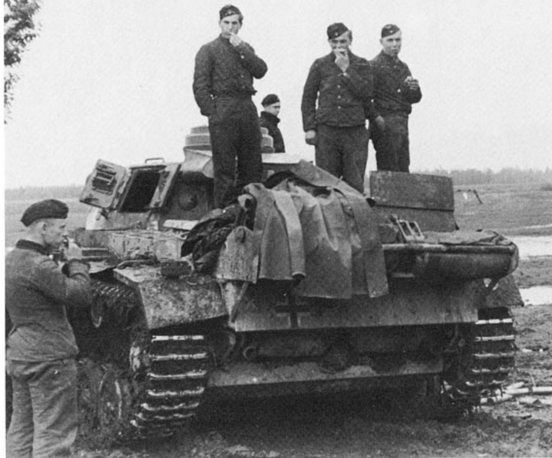
This overall Dark Yellow PzKpfw III Ausf L of 5.PzDiv carries the division sign in Yellow Ochre against a patch of Dark Gray on the hull tail plate next to the national insignia. This vehicle has been modified with a field-made stowage rack welded to the rear hull.
